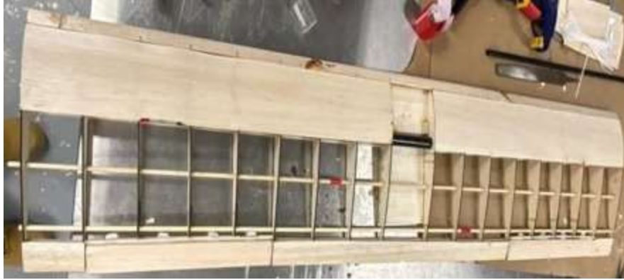
Figure 53: Assembled wing prior to MonoKote.
