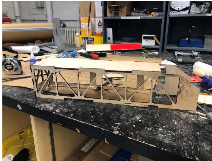
Figure 54: Partially assembled fuselage with lightening holes.
