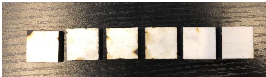
Figure 46: Test cuts of balsa plywood using different settings.
