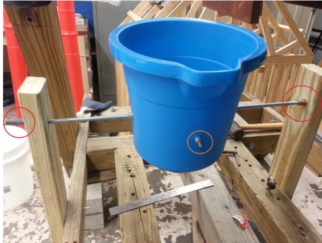
Figure 21 - Completed tipping bucket mechanism
