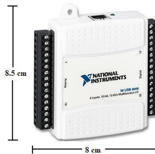
Figure 11 – National Instruments DAQ and Specifications
