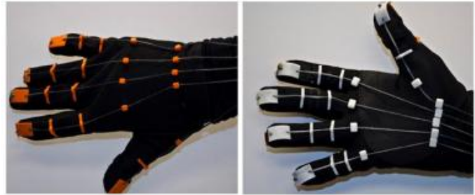
Figure 14. Bowden cable actuated rehabilitative glove [31]
