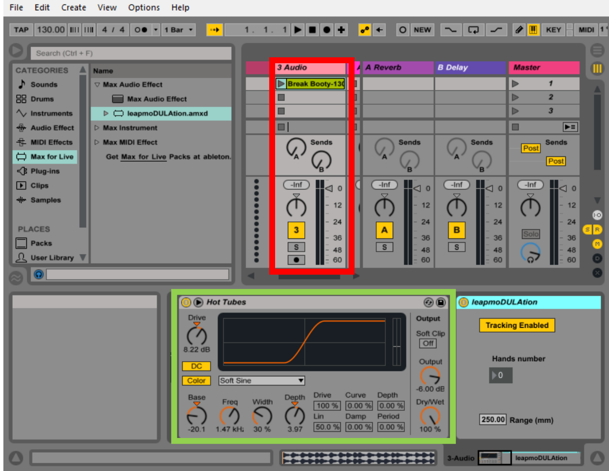
Figure 25. Ableton Live 9 scene. Highlighted in red is an audio clip. Highlighted in green is a saturator audio effect
