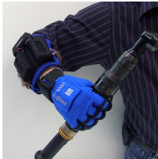
Figure 5. Pneumatic continuum actuator glove
