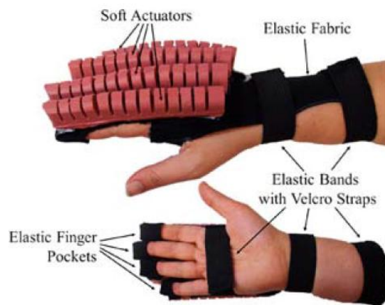
Figure 13. Pneumatic continuum actuated rehabilitative glove [32]
