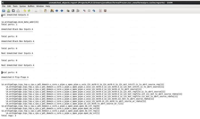
Figure 4: Archipelago Unmatched D Flip-flops in A Design shows three main registers that are appearing only in the A Design. Below these three registers are other registers that are affected by these registers being unmatched. These registers kept the verification from coming back clean and thus preventing the project from moving forward.
