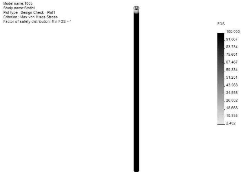
Figure A.1: Finite element stress analysis of bearing rod using cosmos
