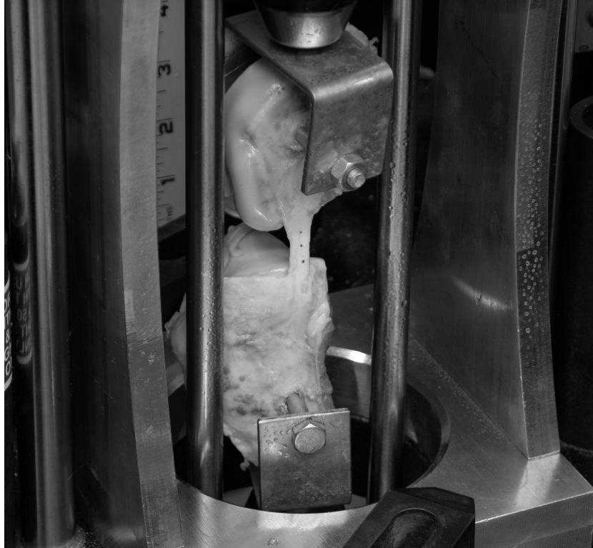
Figure 2.4: Photograph of gripping method using brackets
