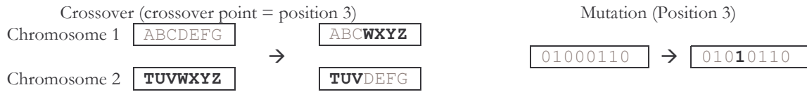
Figure 2.6: Crossover and Mutation in a Genetic Algorithm
