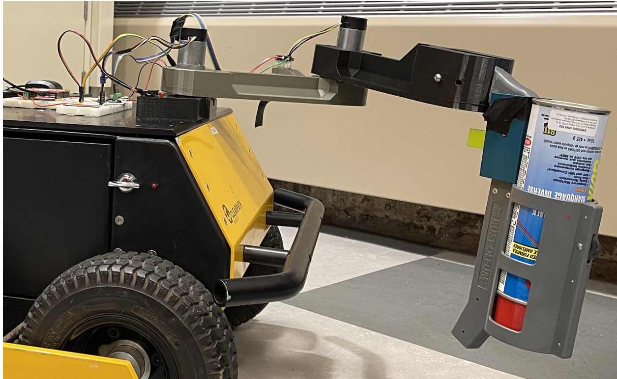
Figure 5: Spray Arm attached to robot
