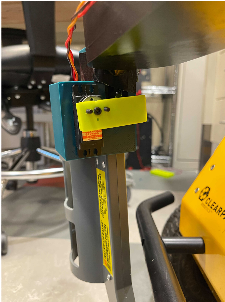
Figure 10: Spray Actuation System
