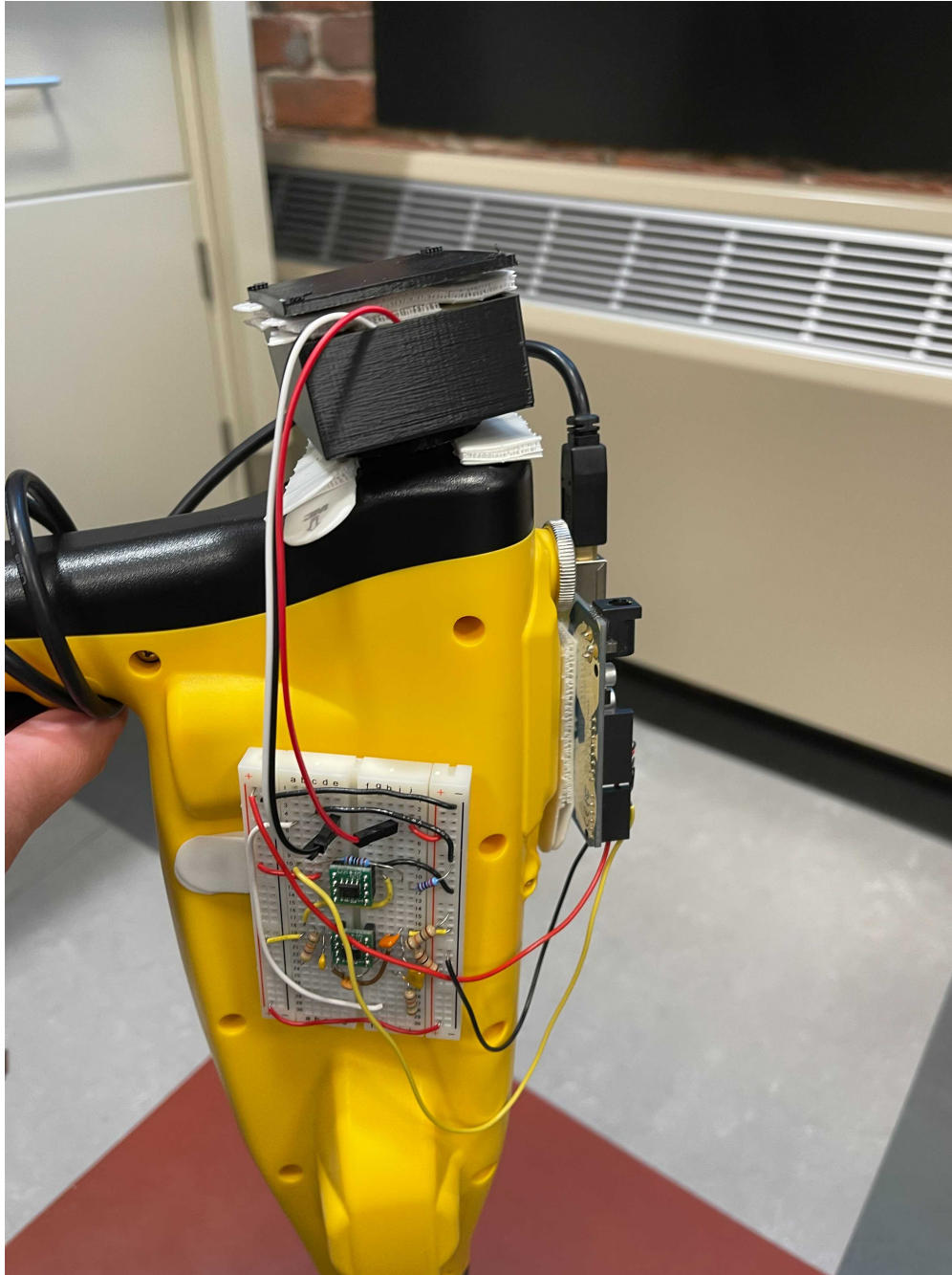
Figure 4: Circuit and Microphone Mounted to Cable Detector
