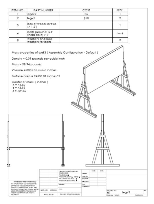
If we consider an adult pushing with a force at a height of 5', the force required to tip the system requires a force of torque<sub>gravity</sub> / sin(angle of moment arm and horizontal) / (moment arm<sub>pushing</sub>) = 2996 ft-in / 67" / sin(63.4 degrees) = 50 lb-f. We decided this was a reasonable expectation of safety. 25
