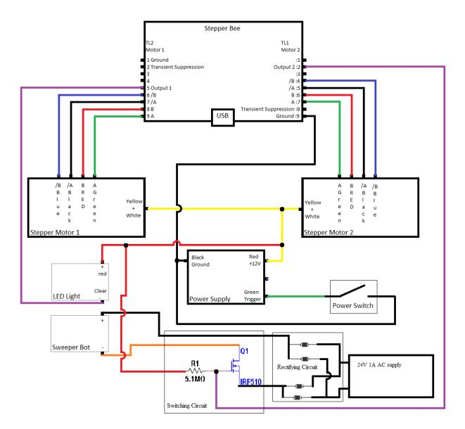
The last thing that needed to be made was the wiring harness that would connect the steppers to the Stepper Bee control board. The wiring harness was made from 14 gauge wire that 31
