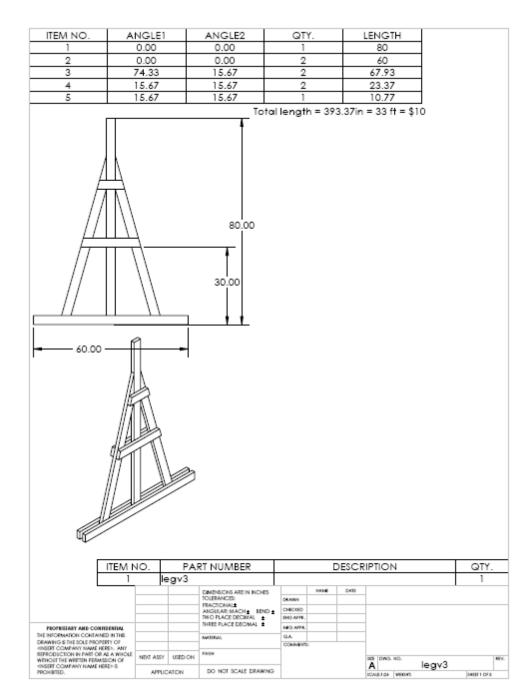
To ensure that the system was safe, we decided to do a few rudimentary calculations on the system. With a total mass of about 100 lbs and some simple trigonometry and physics, we were able to determine the force needed to knock over our board. The torque generated by the weight of the system is (board weight) \* sin(90 - (angle of moment arm and horizontal)) \* (moment arm distance) = (100 lb-f) \* sin(90 - 56.3) \* (54) = 2996 ft-in.
