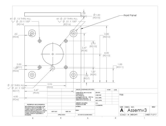
The system was refined until it was simple enough that it could be machined using only drilling operations, and the entire system was fitted together and attached to the wooden board through the specified bolt pattern.
