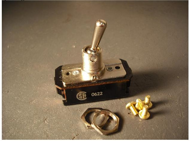
We were able to determine that using the kinetic energy of the system itself, we would be able to trigger a switch similar to the one pictured above. Such a setup however required a particular geometry however, to reach over the body of the upper bracket and contact the switch correctly.
