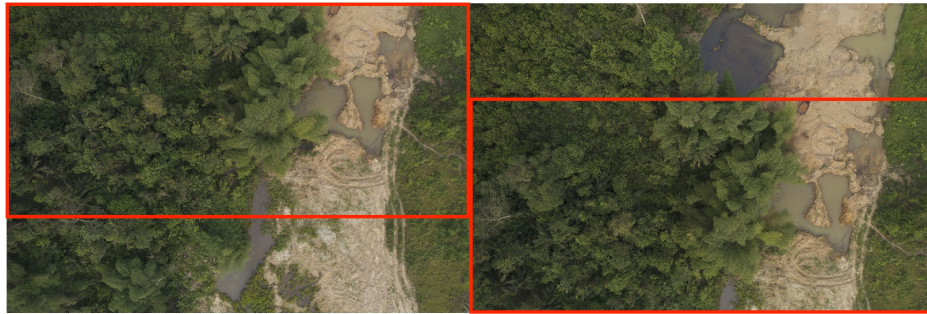
Figure 16: Two consecutive photos in their original state, with the red boxes indicating the overlapping areas.
