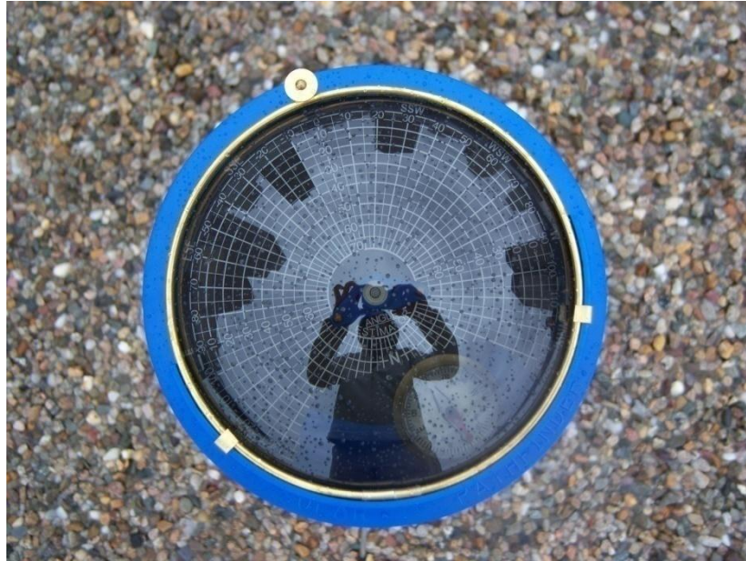
Figure 3: Taking a Reading with the Solar Pathfinder on Top of Boston's City Hall
