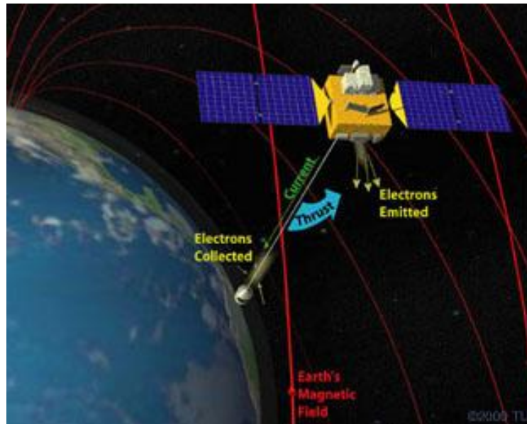
FIGURE 3: PRINCIPLE OF ELECTRODYNAMIC TETHER PROPULSION 5
