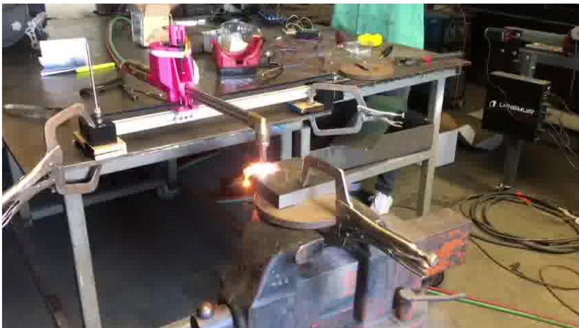
Figure C.5: Picture of Second Cutting Test, close distance to metal created bad cut quality
