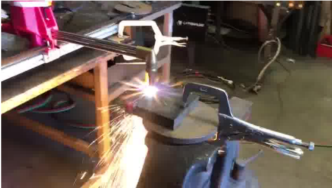
Figure C.8: Picture of Third Cutting Test, cutting quality improved
