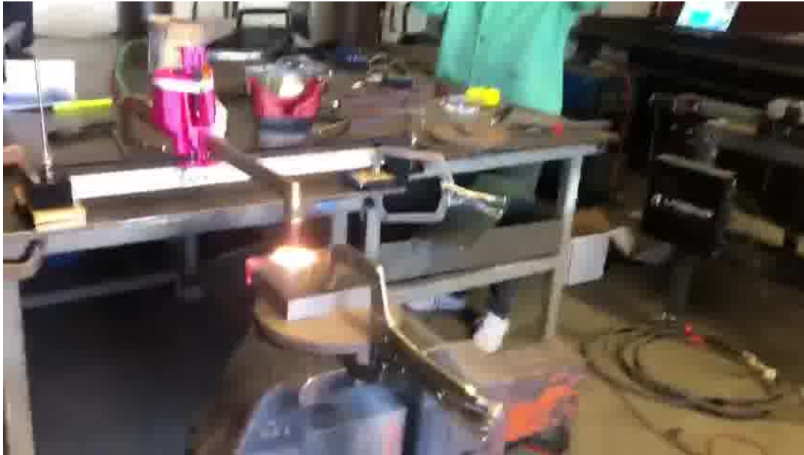
Figure C.6: Picture of Second Cutting Test, close distance to metal created bad cut quality
