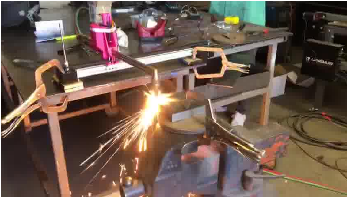
Figure C.2: Picture of First Cutting Test, Rough cutting at beginning
