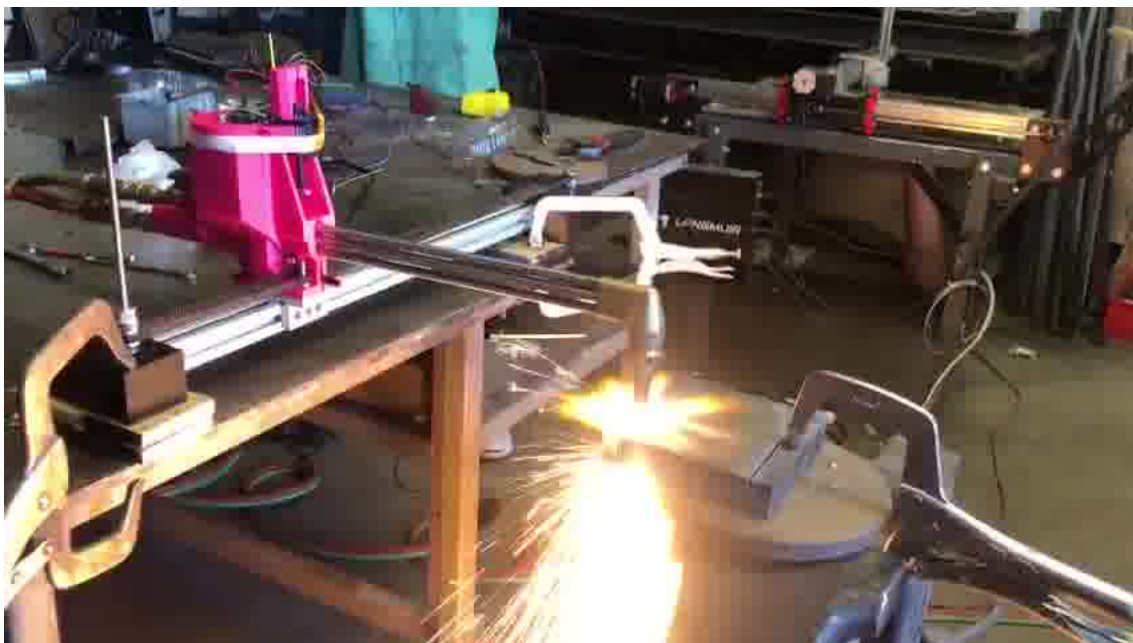
Figure C.11: Picture of Fourth Cutting Test, notice constant star pattern
