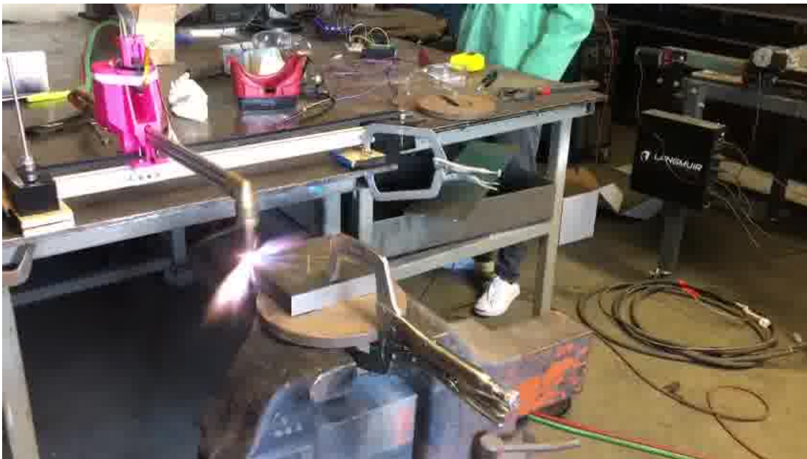
Figure C.1: Picture of First Cutting Test, Rough cutting at beginning
