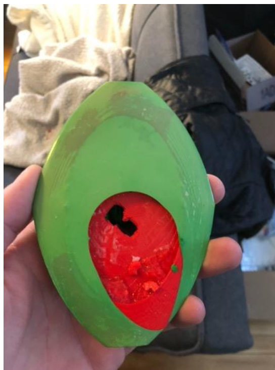
Figure 3-22: Second Pouch Iteration Airsoft Rifle Test
