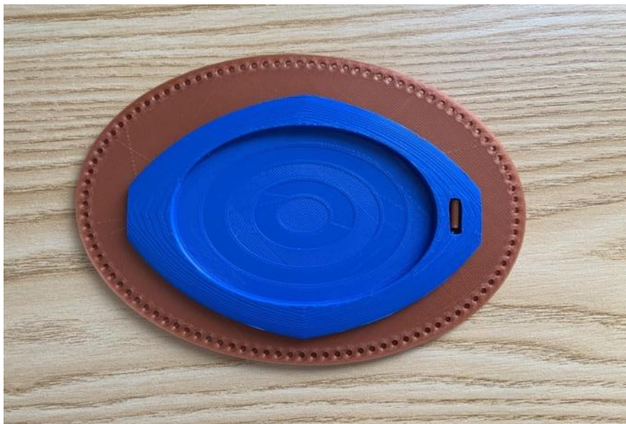
Figure 3-29: 3D Printed Pouch and Fin Assembly
