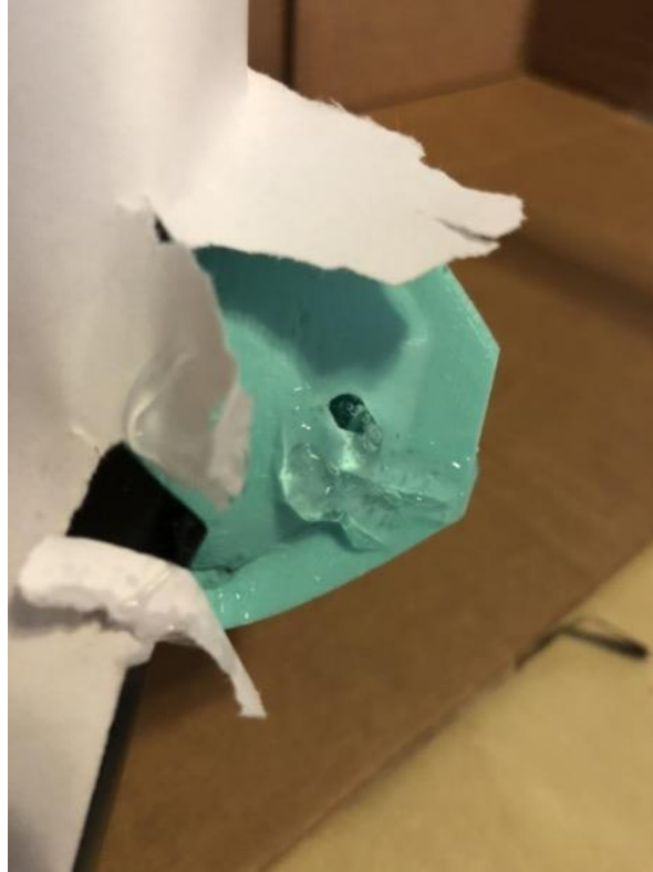
Figure 3-10: Airsoft Rifle Trial on Silicone Pouch
