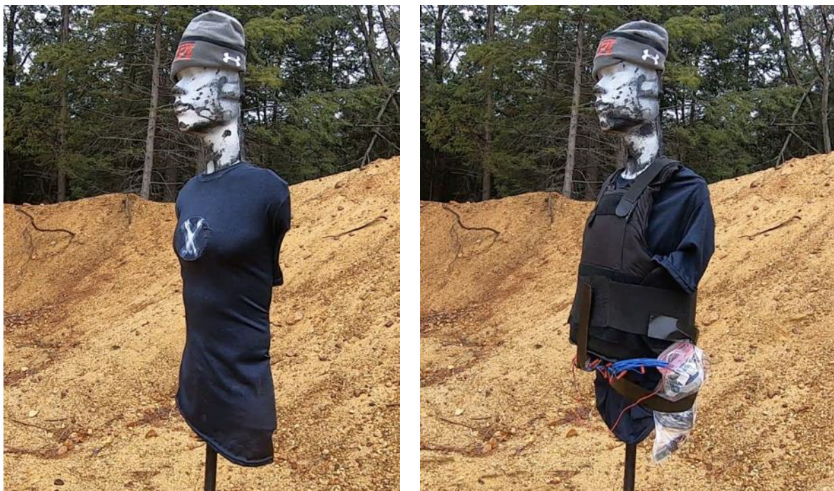
Figure 4-2: Gel Pouch Testing Setup (Left) and Wire Grid Testing Setup (Right)
