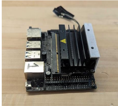
Figure 36: Jetson 1 with Plate to hold in SD Card
