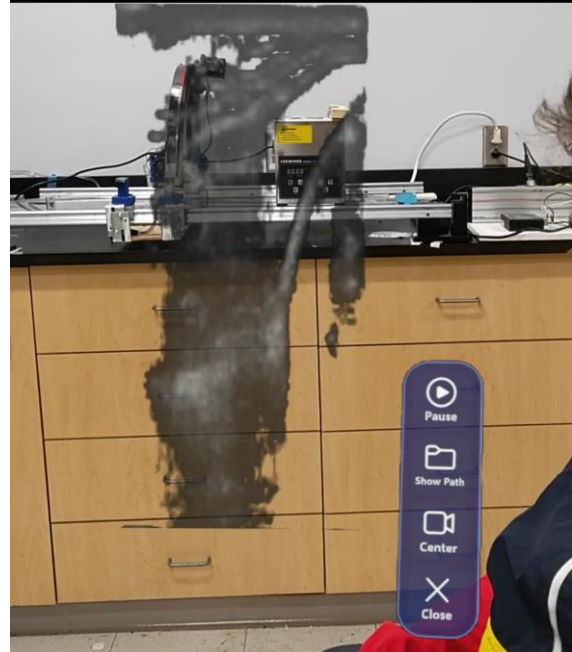
Figure 6: The blue interface on the right appears after the user raises either hand, palm facing user. The image to the left is an ultrasound frame of the patients forearm. It should be noted that the video rendering of the HoloLens, when screen recording, eliminates the black background associated with the ultrasound images. However, when viewing the images in the HoloLens 2, the black background is still present.
