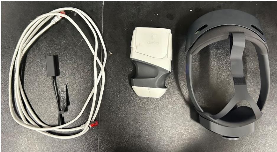
Figure 3: The photo above displays the hardware in which our team used to integrate, aside from our own personal computers, ultrasound imaging into augmented reality. On the left, the white wire and black adapter are used to as a wired connection to send data from Unity to the HoloLens 2 headset through the holographic remoting application. In the middle is the Clarius wireless ultrasound probe. Finally, on the right is the Microsoft HoloLens 2 augmented reality headset.
