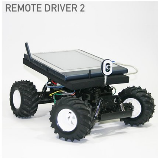
Fig 3.1-1: A robot built on a remote controlled car chassis.
