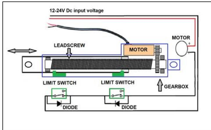
Figure 1: DC Electrical Linear Actuator Schematic
