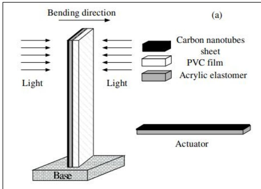
Figure 7: Diagram of Process 1 CNT film actuator (Lu, Panchapakesan, 2005)
