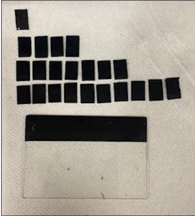
Figure 9: Process 2 CNT actuator test strips
