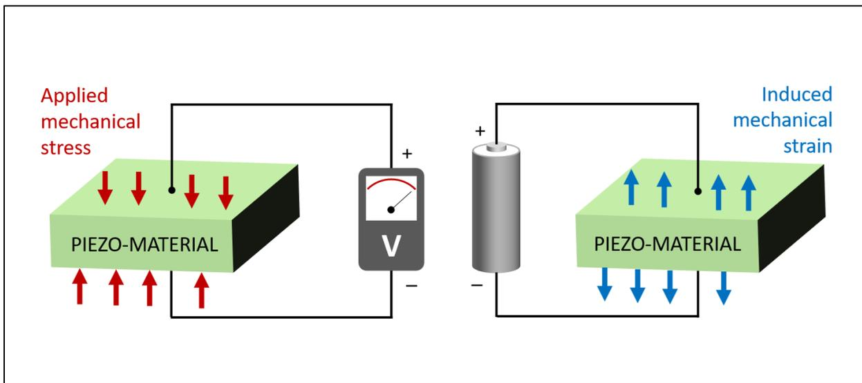
Figure 3: Schematic of Piezoelectric and Inverse Piezoelectric Effect
