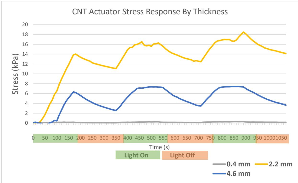
Figure 14: Stress plot comparison of all CNT actuators
