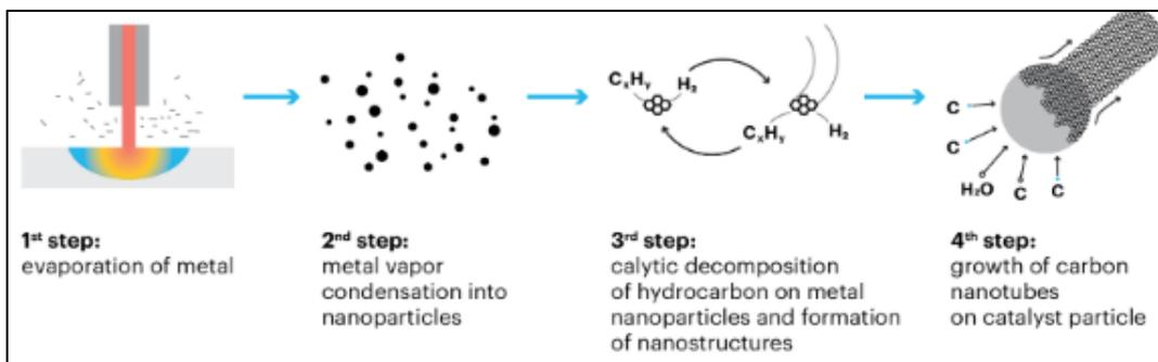
Figure 6: Key Steps in the standard CVD production process (Filchakova & Saik, 2021)
