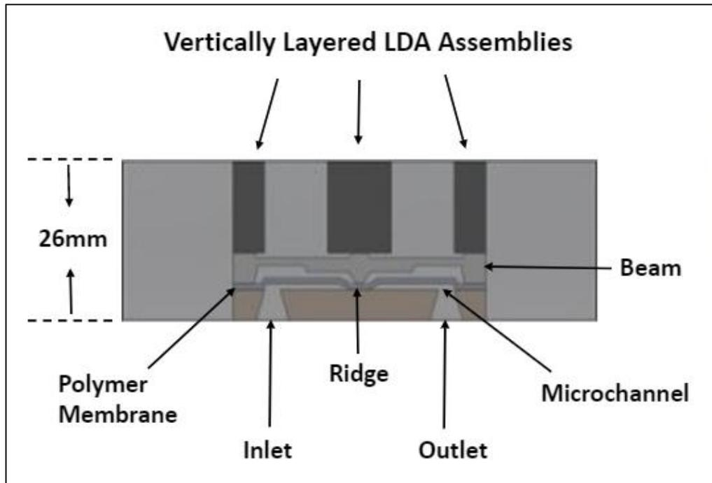
Figure 15: Light actuated microvalve prototype design
