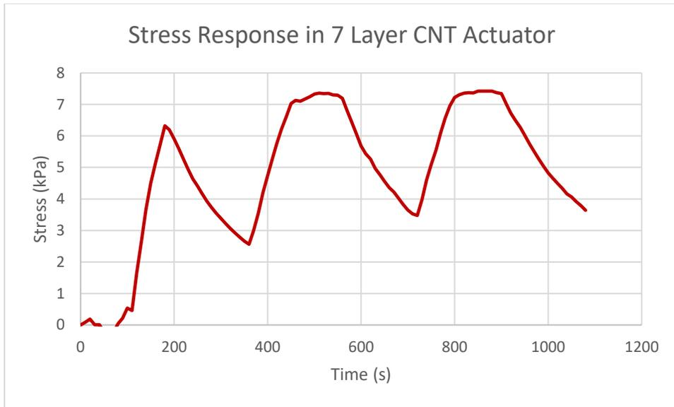
Figure 12: 7 Layer CNT actuator stress plot
