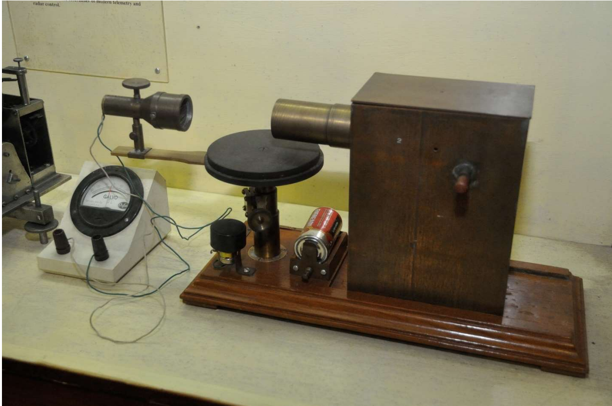
Figure 5. A photograph of Bose's 60 GHz emitter and receiver at the Jagadish Chandra Bose Museum in Kolkata [25].
