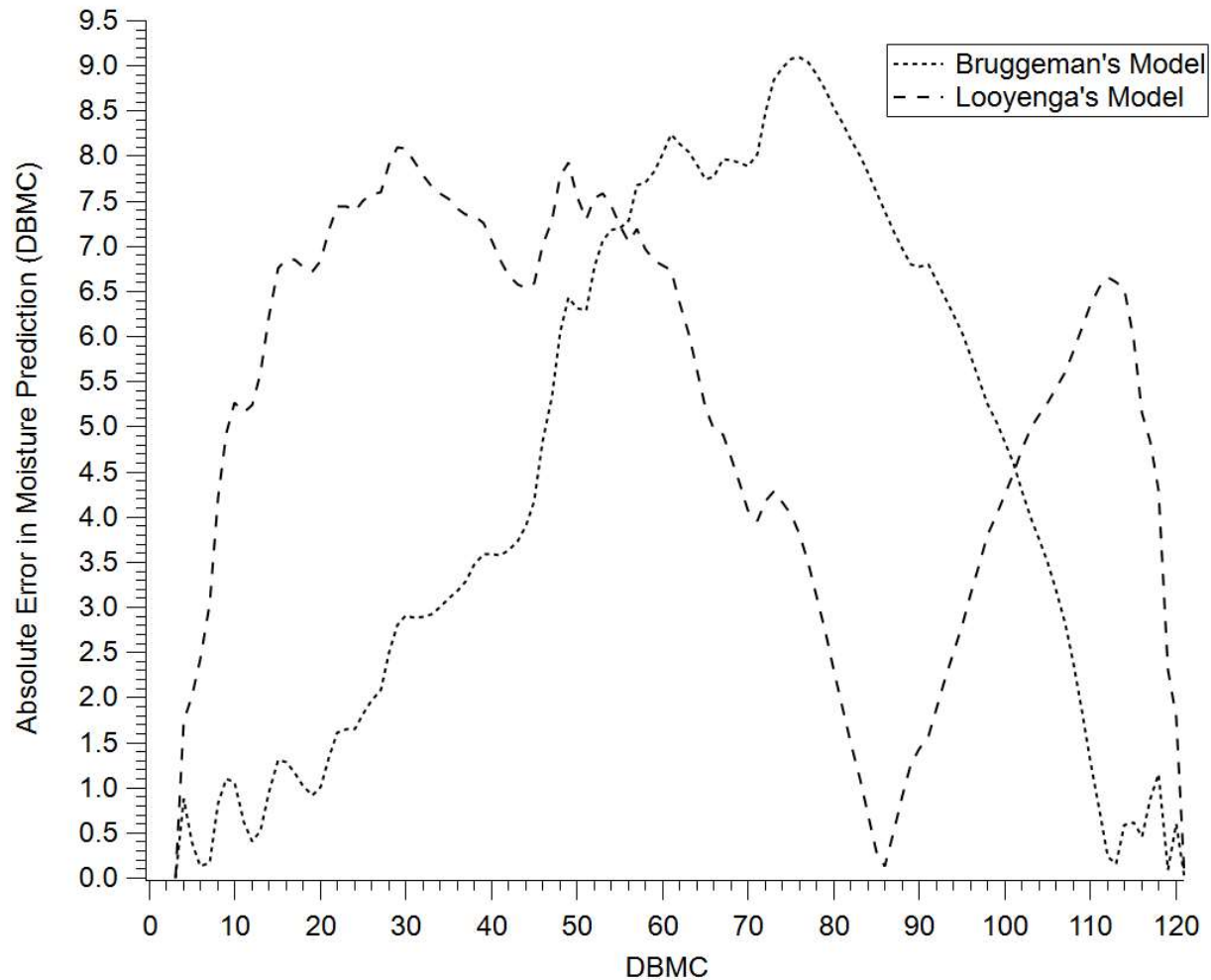
Figure 73. The absolute error in the moisture content predictions from the two models, showing that Bruggeman's model has a lower average error.
