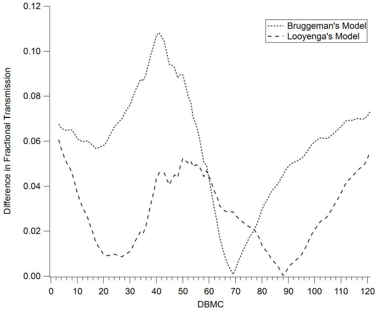
Figure 70. The absolute difference between the predicted fractional transmission through a sample as a function of moisture content from Bruggeman's and Looyenga's models and the experimental data at 300 GHz.
