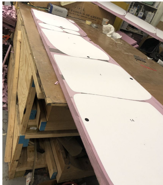
Figure 61: Contours glued to foam board
