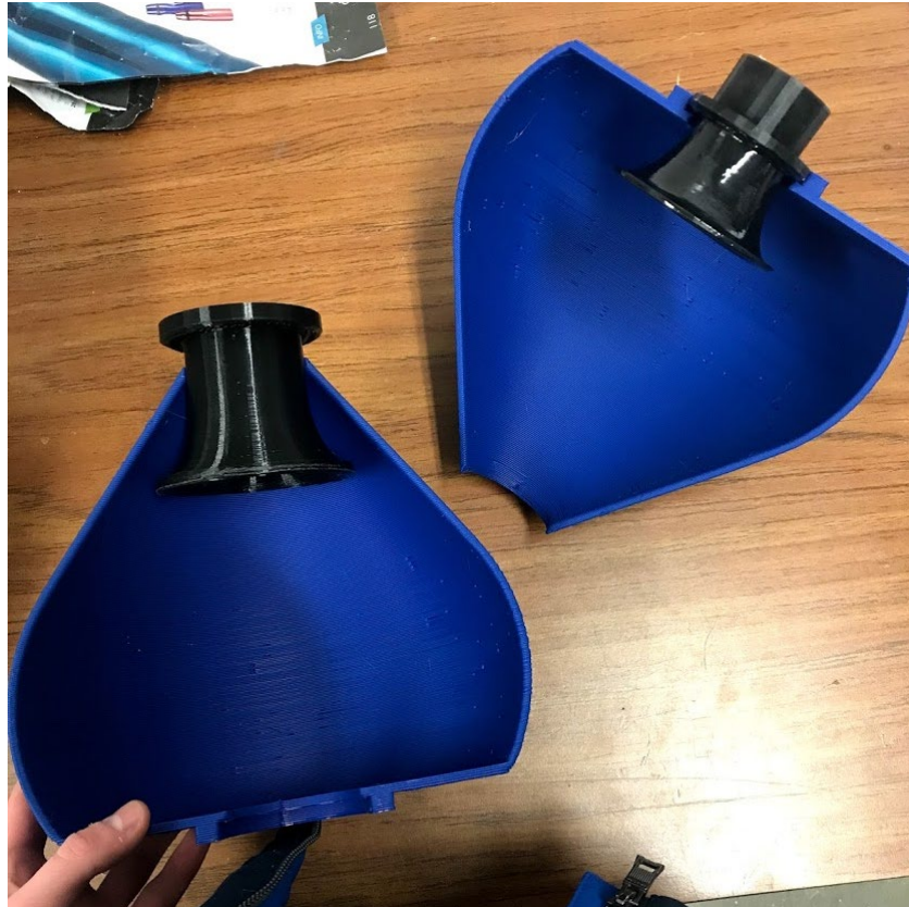
Figure 14: 3D printed intake system
