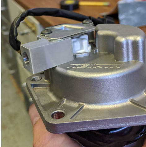
Figure 28: Suzuki RMZ 450 Pump Assembled with CNC Machined Adapter
