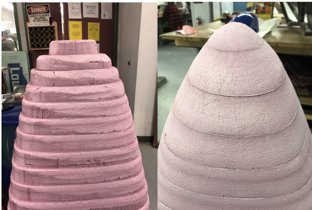
Figure 64: Mold sanding in progress (left) and complete (right)
