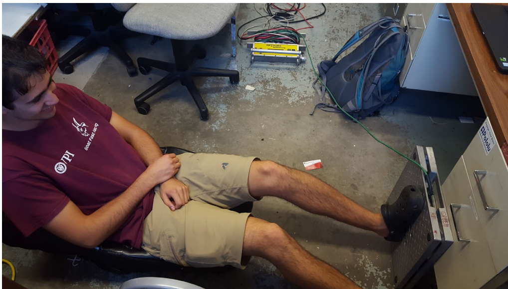
Figure 38: Test procedure for determining maximum braking force
