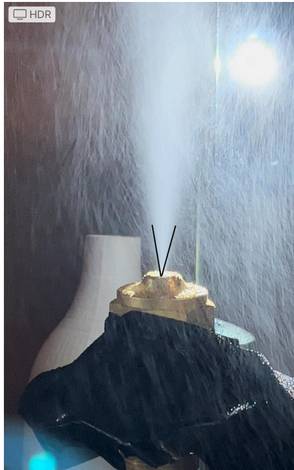
Figure 62: 34 Degree Angle of Dispersion at 30 psi
