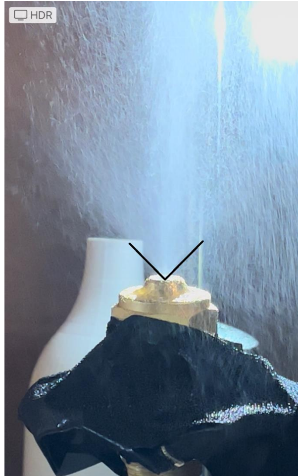
Figure 63: 74 Degree Angle of Dispersion at 30 Psi
