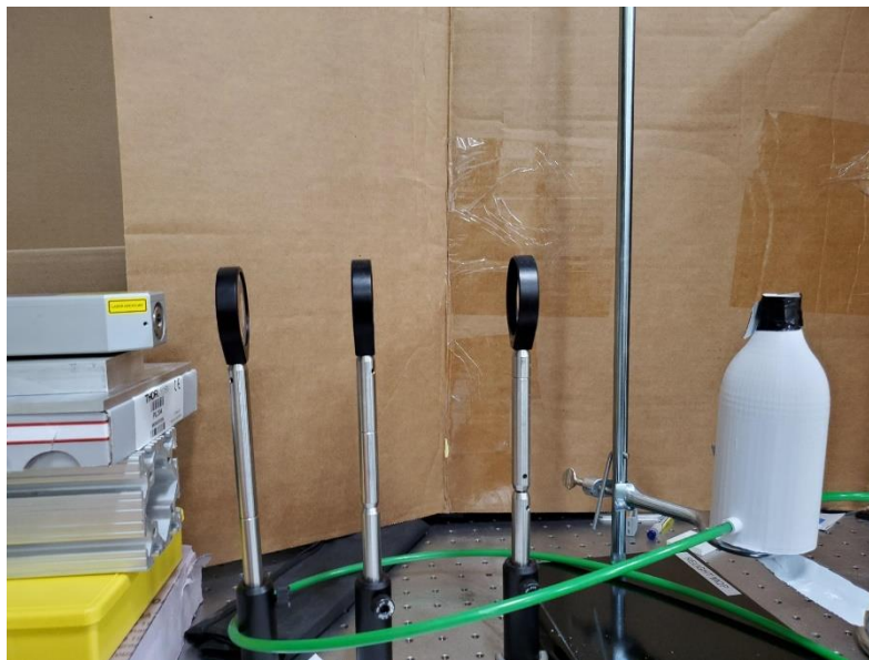
Figure 56: Experimental Setup Featuring the Burner and Laser, Focused by 3 Lenses
