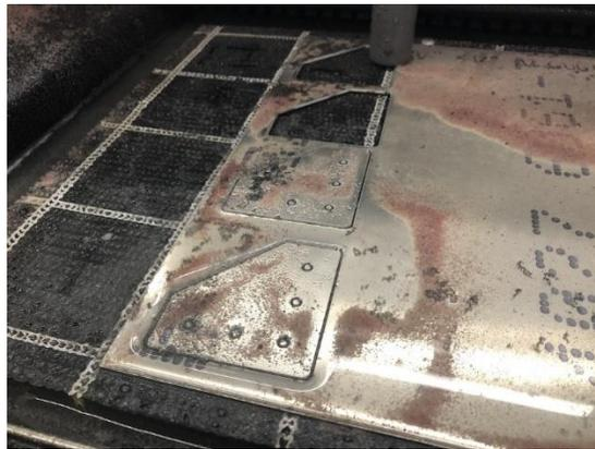
Figure 63. Triangle Brackets in Wazer Waterjet.
