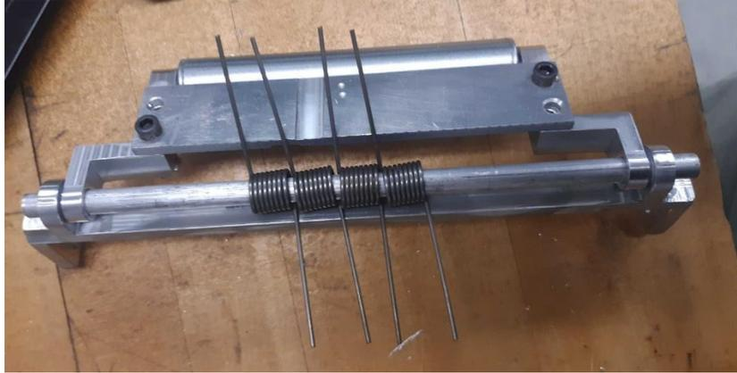
Figure 44. Storage & Deposit Conveyor Belt Tensioner.
