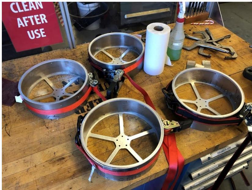
Figure 66. Wheel Fixturing for Epoxied Joining Plates.
