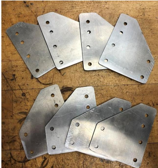
Figure 64. Motor Mount Brackets.
