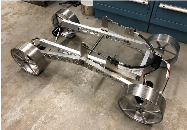
Figure 60. Assembled Chassis Prior to Mounting Wheel Grousers.
