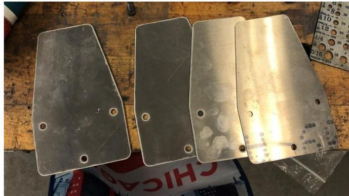
Figure 69. Mounting Brackets for Suspension Cable Mounting Clamp.
