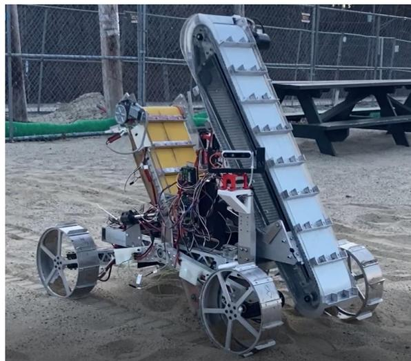
Figure 119. Robot in Depositing Configuration.
