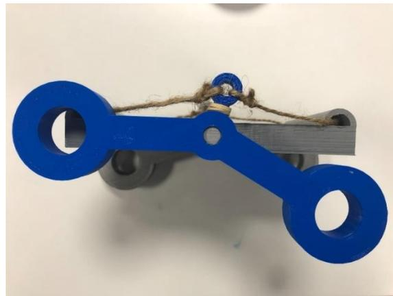
Figure 15. Rocker Pull Cable Prototype.
