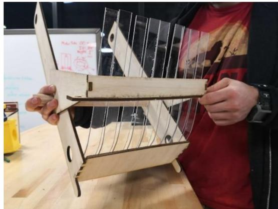
Figure 41. Storage & Deposit Fingers Prototype.
