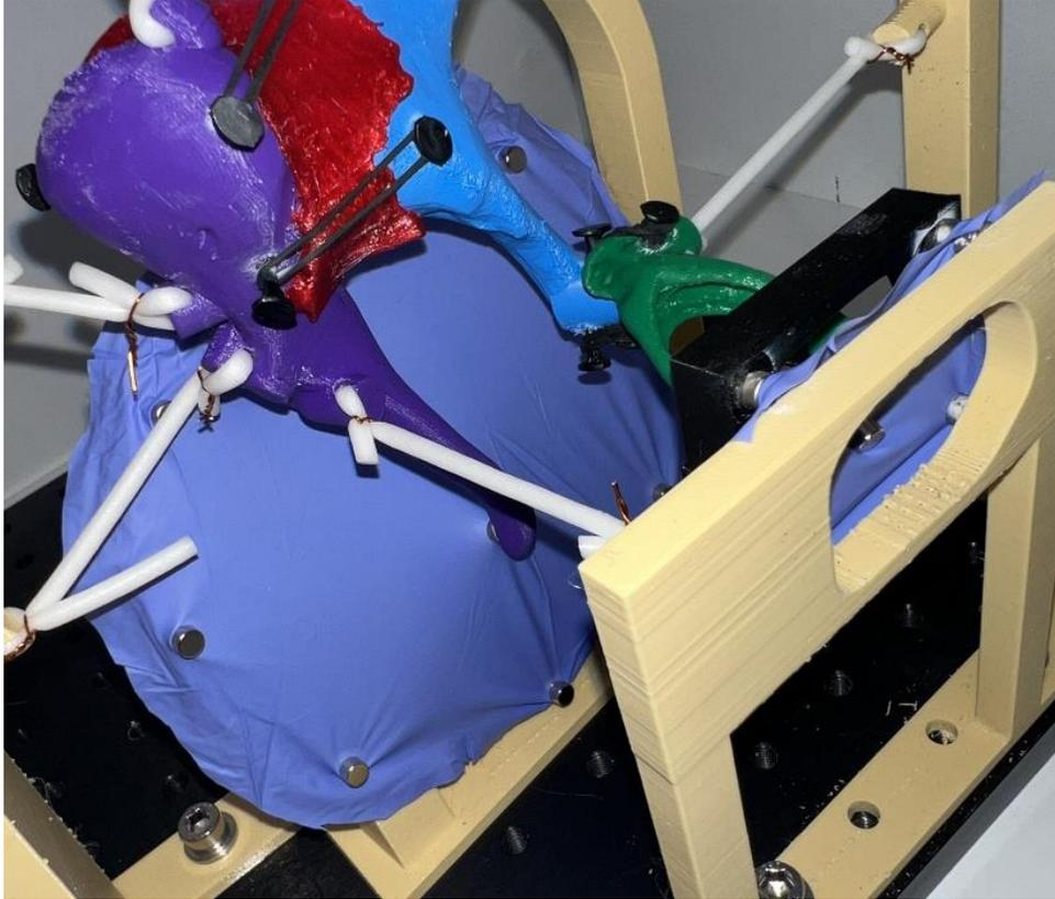
Fig. 4.29. Ear canal membrane connection with magnets
