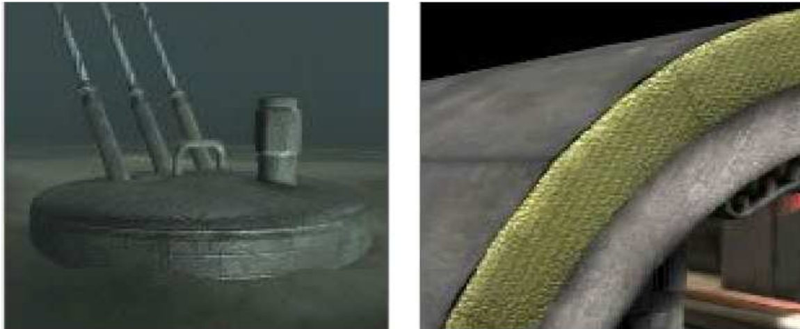
Figure 10: Left: Anchored Tethers, Right: Foam Coated Gasket for Lining Tube
