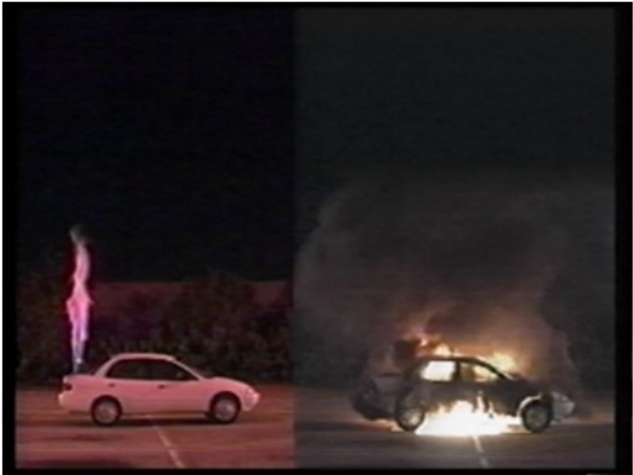
Figure 3 Hydrogen vs. Gasoline; 1 minute after ignition (Swain, 2001)
