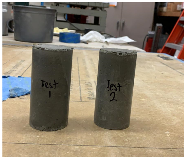
Figure 40: Cylinders Following Manufacturer's Mix Design
