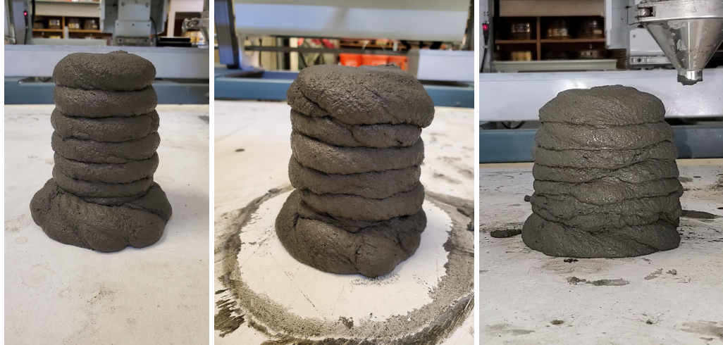
Figure 42: 2" x 4" Inch Test Cylinders Using Final Mix Design
