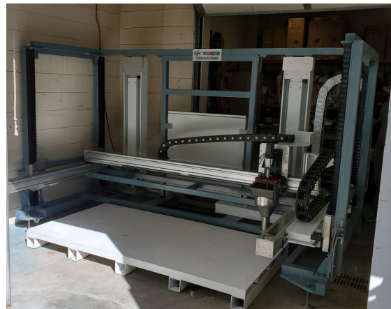
Figure 2: Gantry 3D Printer used in Project
