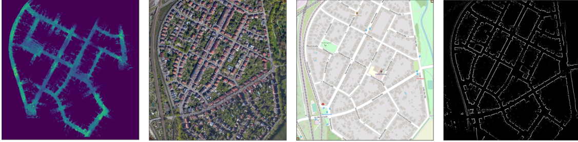
Figure 2.1: Examples of Visual Maps. From left to right: LiDAR map, satellite map, OSM and simulated LiDAR map.
