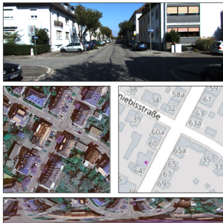
Figure 2.3: Front view camera frame (top), followed by the same area in a satellite map (middle left) and in OSM (middle right). The final image is the polar projection of the satellite crop (bottom).
