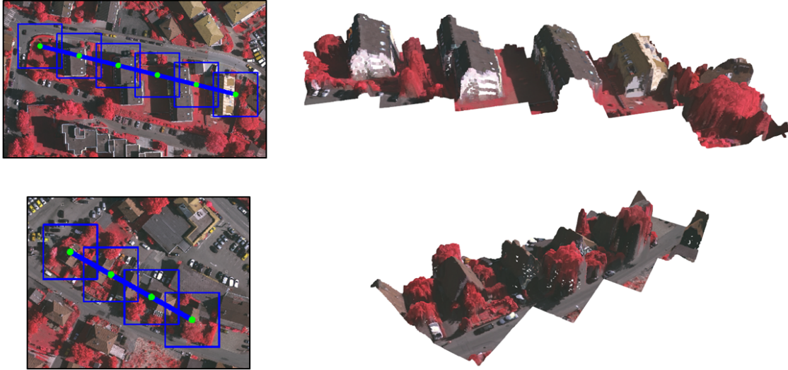
Figure 3.8: 3D reconstructions from simulated UAV flight. From left to right: Positions of the UAV images, Reconstructed 3D scene.
