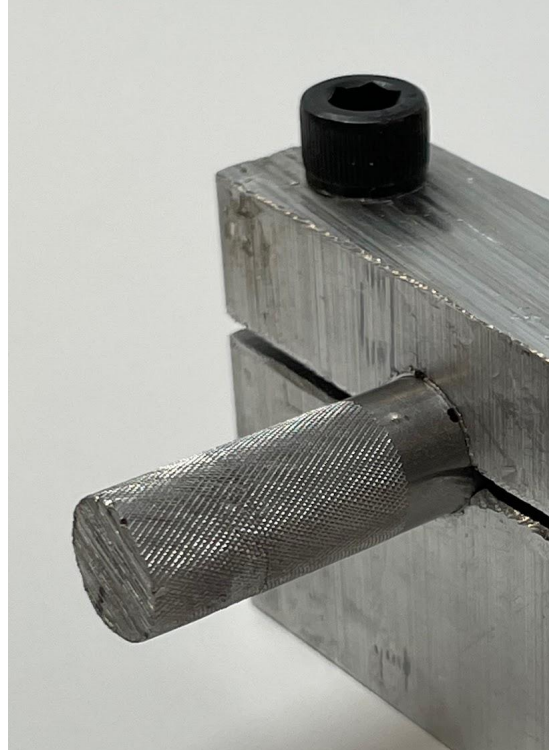
Figure 55: Knurling with Offset Imprints
