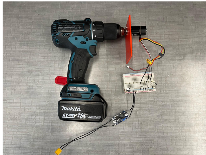
Figure 32: Drill Power Regen Test Setup
