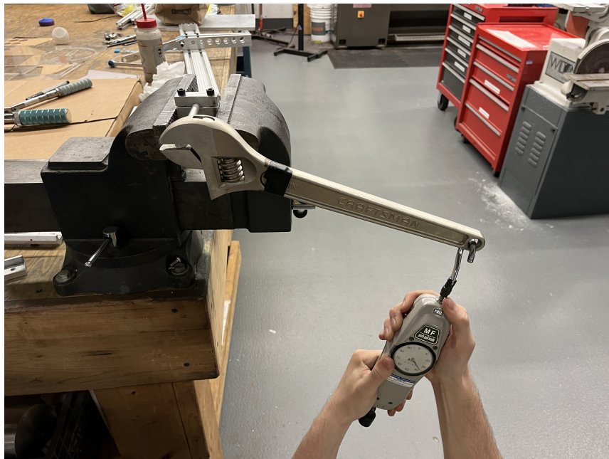
Figure 30: Steel Rod Slip Test Setup
