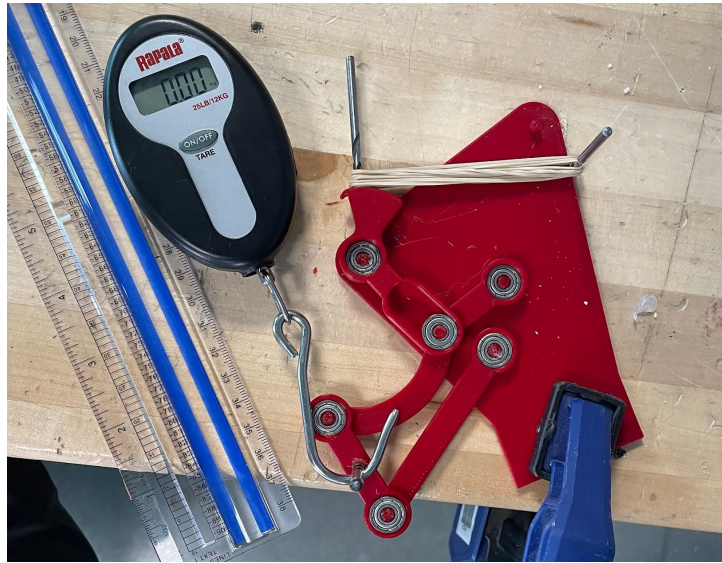
Figure 16: Slider Linkage First Iteration, Testing Setup
