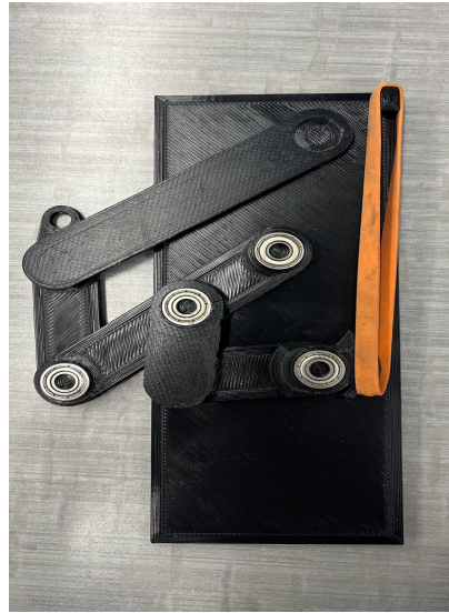
Figure 11: 3D Print of Perpendicular Linkage Concept
