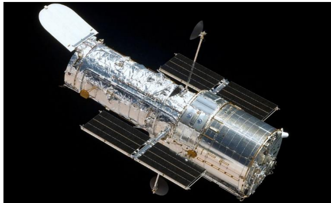
Figure 8: Hubble Space Telescope covered in MLI with an aluminized Teflon outer layer (Wittry, 2009)
