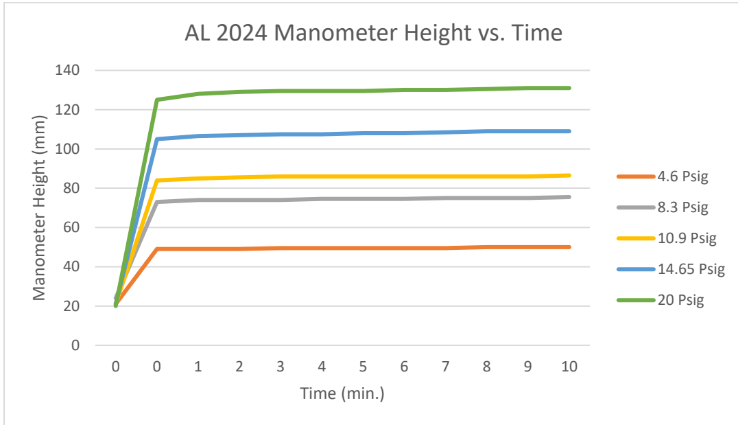
Figure 51: Displacement in manometer fluid height during Al 2024 permeability testing. Note the initial spike in the fluid height.
