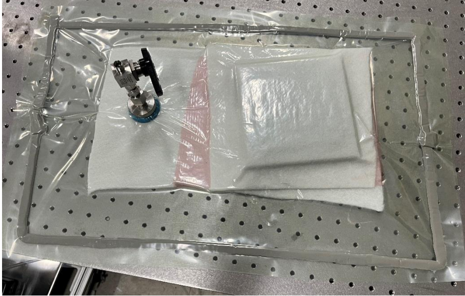
Figure 37: Vacuum sealed bag of 6-ply composite material prior to being oven-cured.
