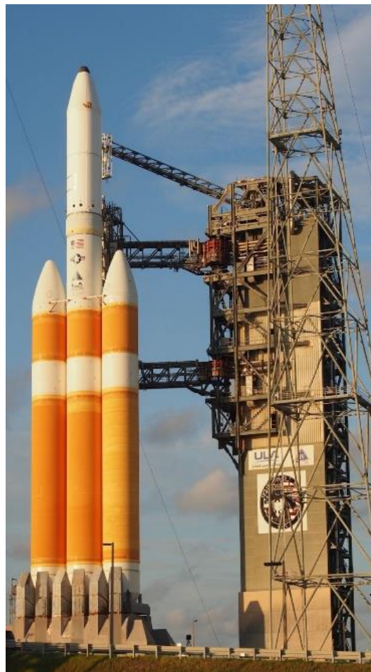
Figure 10: The entirely LH 2 fueled Delta IV Heavy rocket preparing for launch; exhibiting orange foam insulation (Erwin, 2019)
