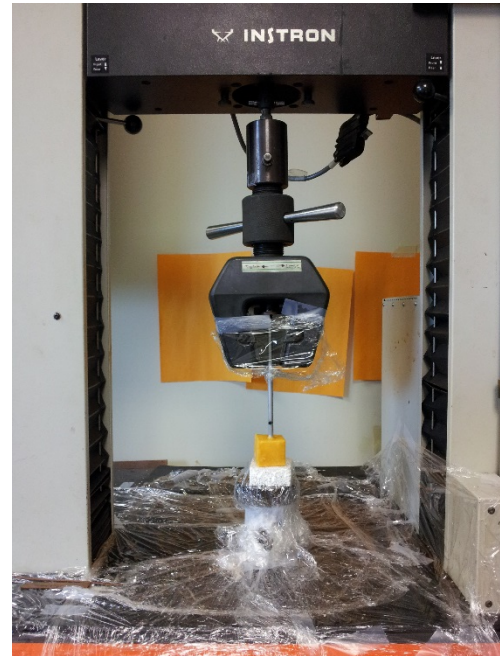
Figure 11. Hardness test set up in Washburn food engineering laboratory.
