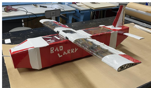
Figure 4.2 Fully assembled and covered glider prototype.
