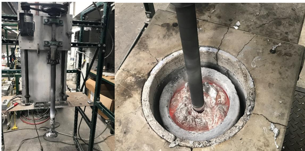
Figure 5.3. Left: Photo of the rotary degasser; Right: Photo of degassing operation
