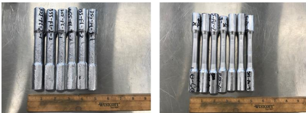
Figure 5.11. Left: Tensile bars from sand molds (one trial). Right: Tensile bars from steel molds (one trial)
