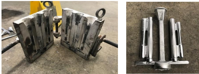
Figure 5.9. Left: Picture of ASTM standard steel mold. Right: The casting from the steel mold
