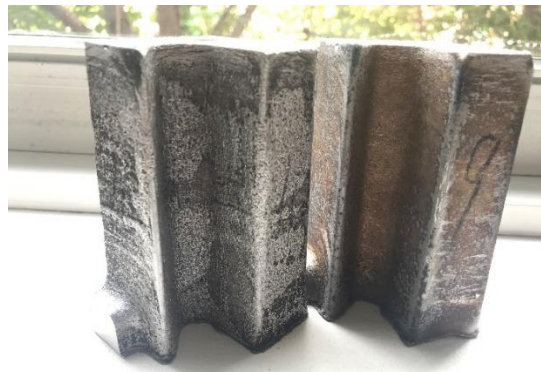
Figure 6.26. Comparison of surface roughness between types of sand mold
