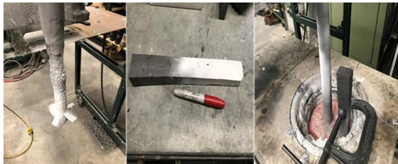
Figure 5.10. Left: The design of the degassing impeller. Middle: The picture of graphite baffle. Right: View of the flux insertion system
