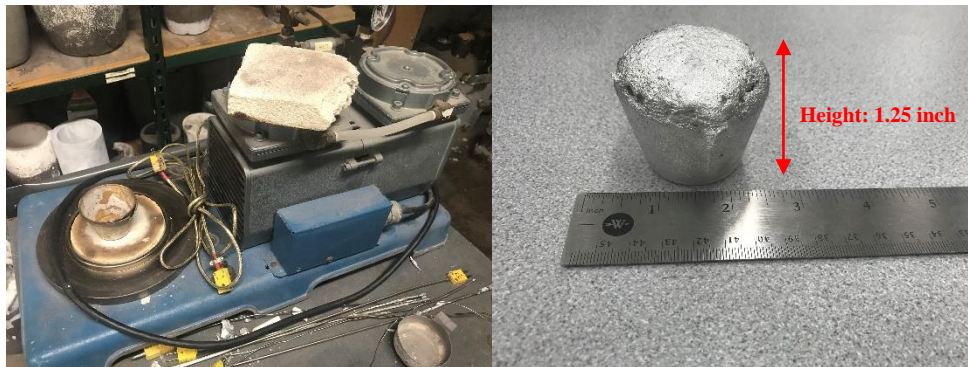
Figure 5.4. Left: The picture of RPT machine; Right: The picture of a RPT sample
