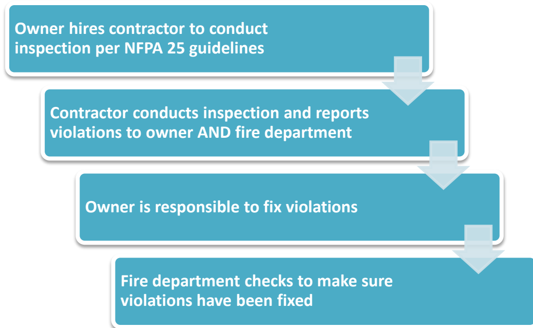
Figure 3: Fire Protection System Inspection Process
