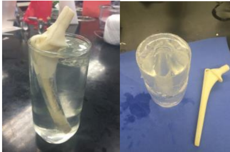
Figure 19: Process for making PDMS molds
