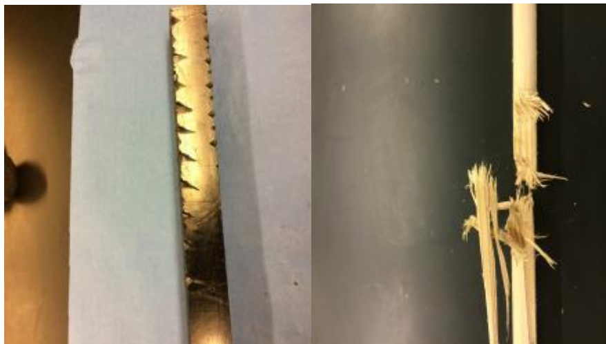
Figure 34: ABS teeth and result of sawing wooden dowel with this instrument
