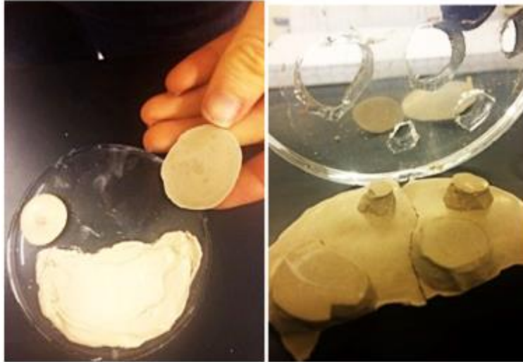
Figure 14: PDMS visual adhesive testing proved to be a success since only dust particles remained on the surface
