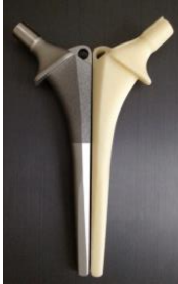
Figure 17: 3-D printed component (right) compared to primary hip stem (left)
