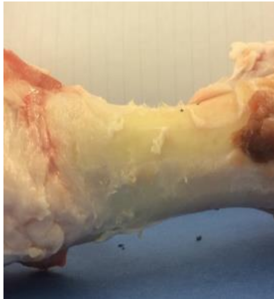
Figure 13: Porcine femur cut with ABS teeth (negligible damage to cortical bone)
