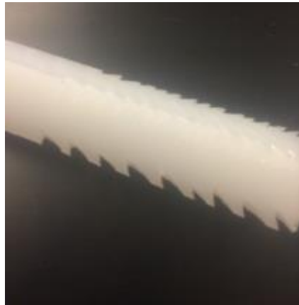
Figure 32: Teeth cut into UHMWPE rod to test on wooded dowels and bovine femur for a proof of concept
