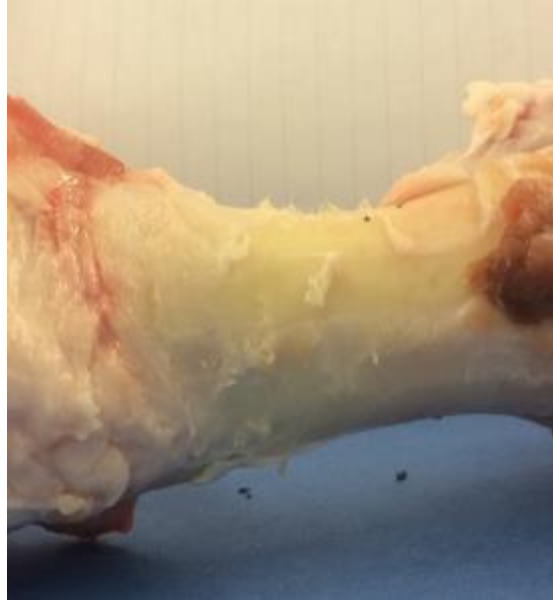
Figure 35: Porcine femur cut with ABS teeth (negligible damage to cortical bone)
