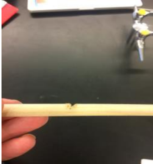
Figure 33: Result of cutting wood with UHMWPE formed teeth
