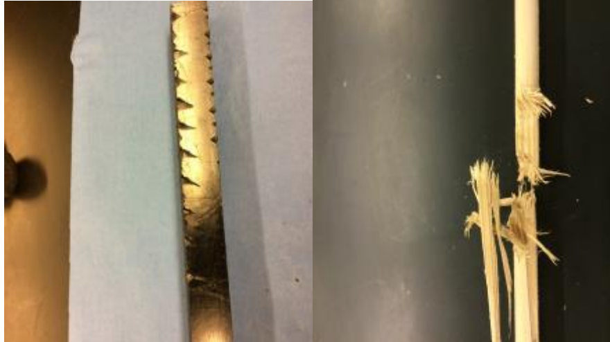
Figure 12: ABS teeth and result of sawing wooden dowel with this instrument
