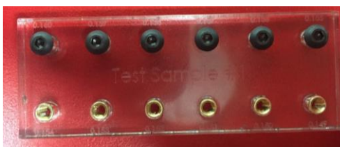
Figure 61: Threaded insert press-fit test
