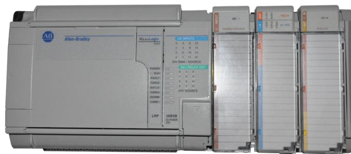
Figure 10: Allen-Bradley MicroLogix 1500 PLC controller with three expansion IO modules (Industrial Automation Control, 2011)
