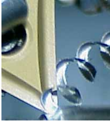
Figure 4-10 TNMP 332K KC850 Insert with 0.03 in. Depth of Cut 0.0046 in/rev Feed Rate
