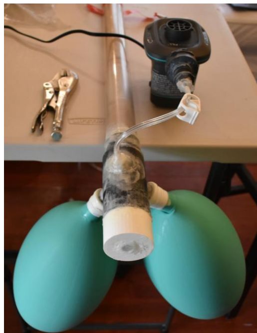
Figure 27: Second Testing Apparatus Two 3L breathing bags were inflated using an air mattress pump.
