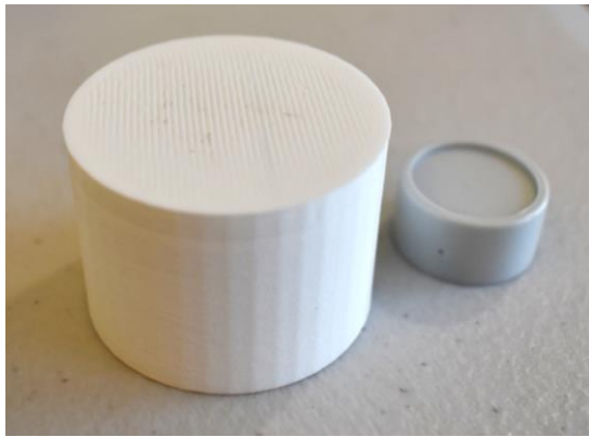
Figure 28: 3D-Printed Outlet Diaphragm (left) compared to the medical grade version (right) The 3D printing process creates ridges in the material, while injection molding does not.
