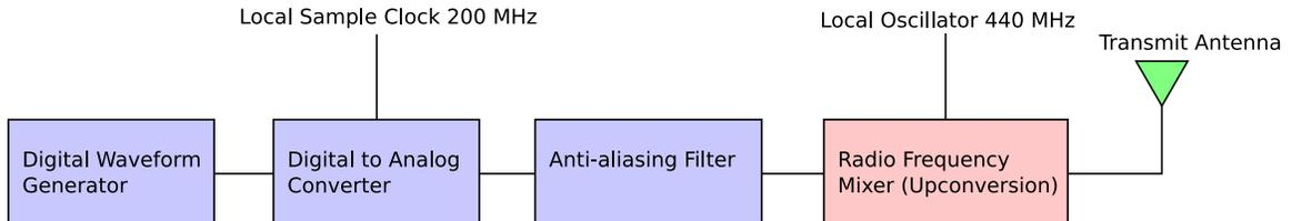
Figure 3.1: Transmitter Block Diagram
