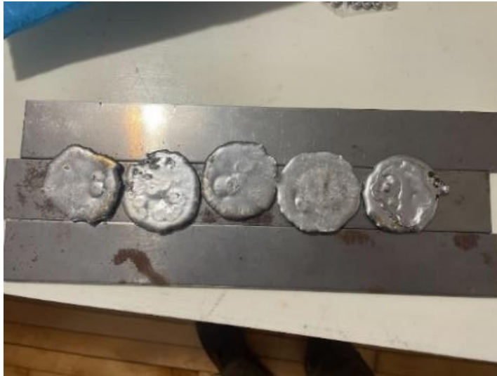
Figure 34: The formed solder pucks and the uncut steel stock
