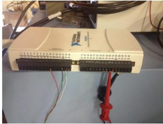
Figure 1: NI-USB 6211 DAQ with load cell leads connected.
