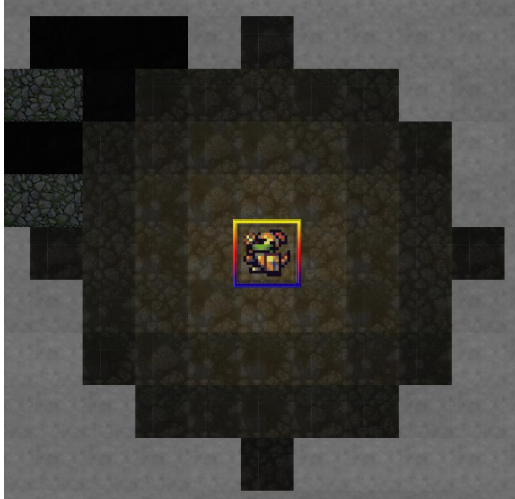
Figure 42. A glow radius is supposed to be a circle, but the result is obviously not. While the source of the light is apparent due to the gradual falloff, the 'corners' of the 'circle' are a result of a square-based rendering engine. Source: Screen capture.
