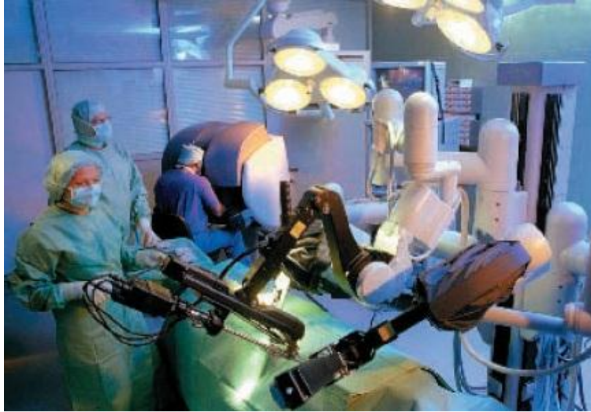
Figure 2.4.1 – Three primary components of the da Vinci system: Surgical cart (most right), vision cart (center arm), and surgeon console (center-left).
