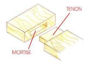
Figure 3.13 The Mortise and Tenon Joint
