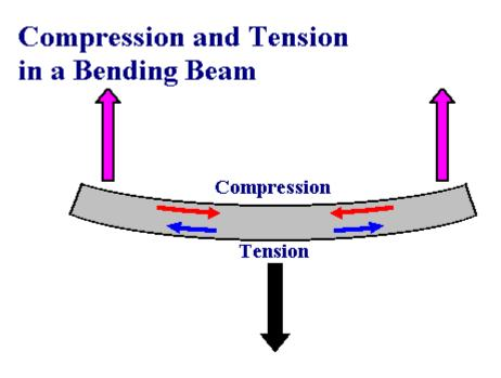
Figure 3.8 This demonstrates how the bridge deck undergoes tension and compression.
