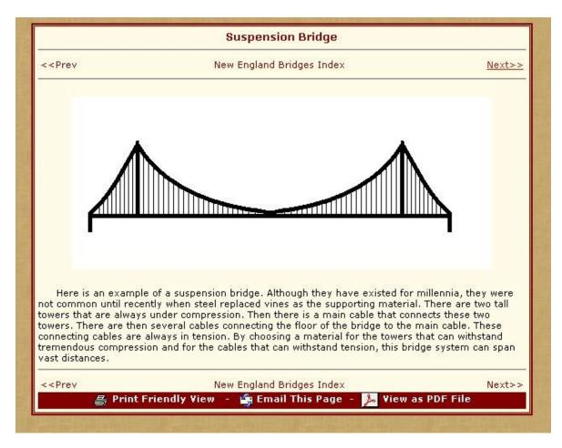
Figure 7.8 Explanation of the suspension bridge.
