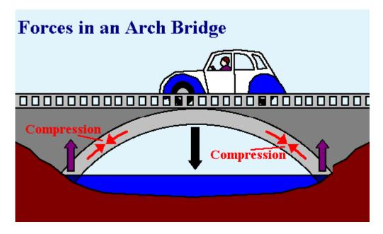
Figure 3.10 Distributed Loading in an Arch Bridge
