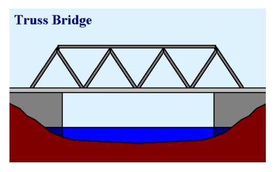
Figure 3.2 The Simple Truss Bridge
