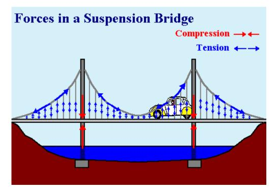
Figure 3.11 Forces in a Suspension Bridge
