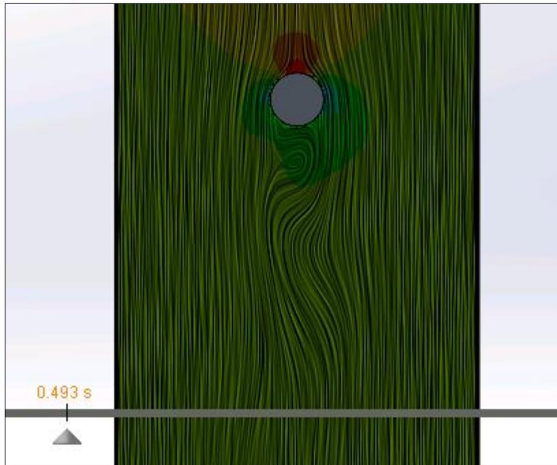
Figure 14: Vortex Street at 0.493 seconds for an Aspect Ratio of 5
