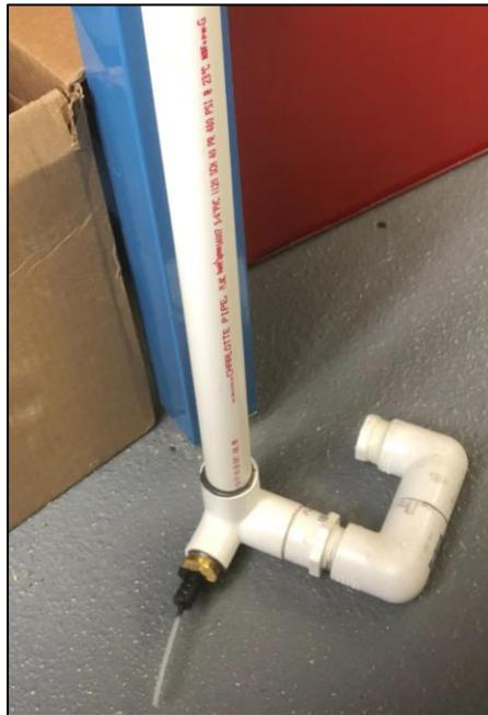
Figure 38: The Pressure Transducer Calibration Pipe Setup
