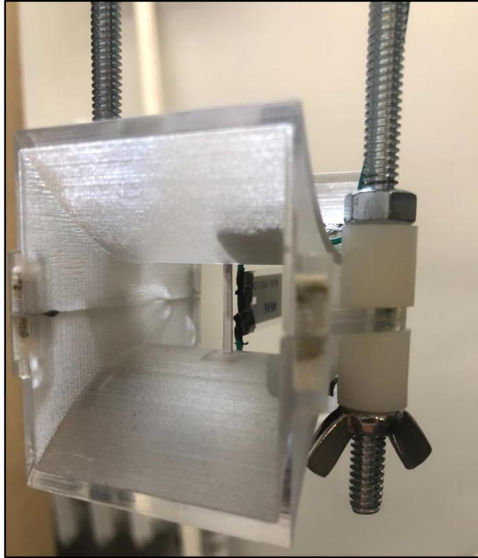
Figure 35: The Fully Manufactured Nozzle
