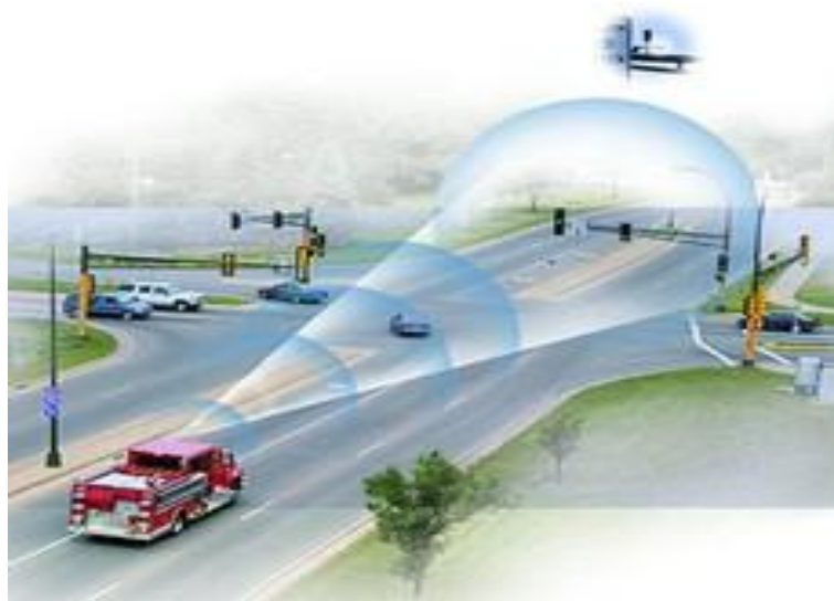
Figure 26: Light-based preemption system (US Department of Transportation [80])
