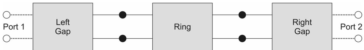
**Fig. 2 Network circuit of planar ring resonator.**
