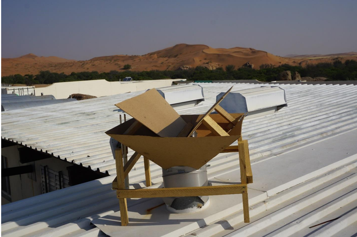
Figure 32. Evaporative cooler prototype
