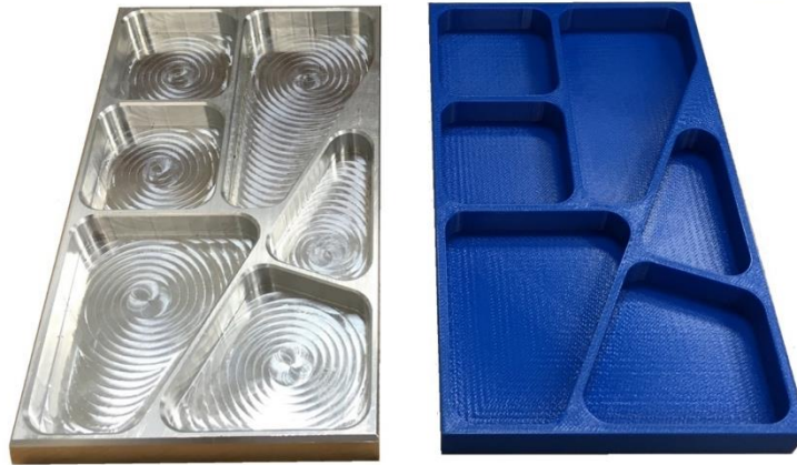
Figure 1: Subtractive manufacturing (left) and Additive manufacturing (right) 1
