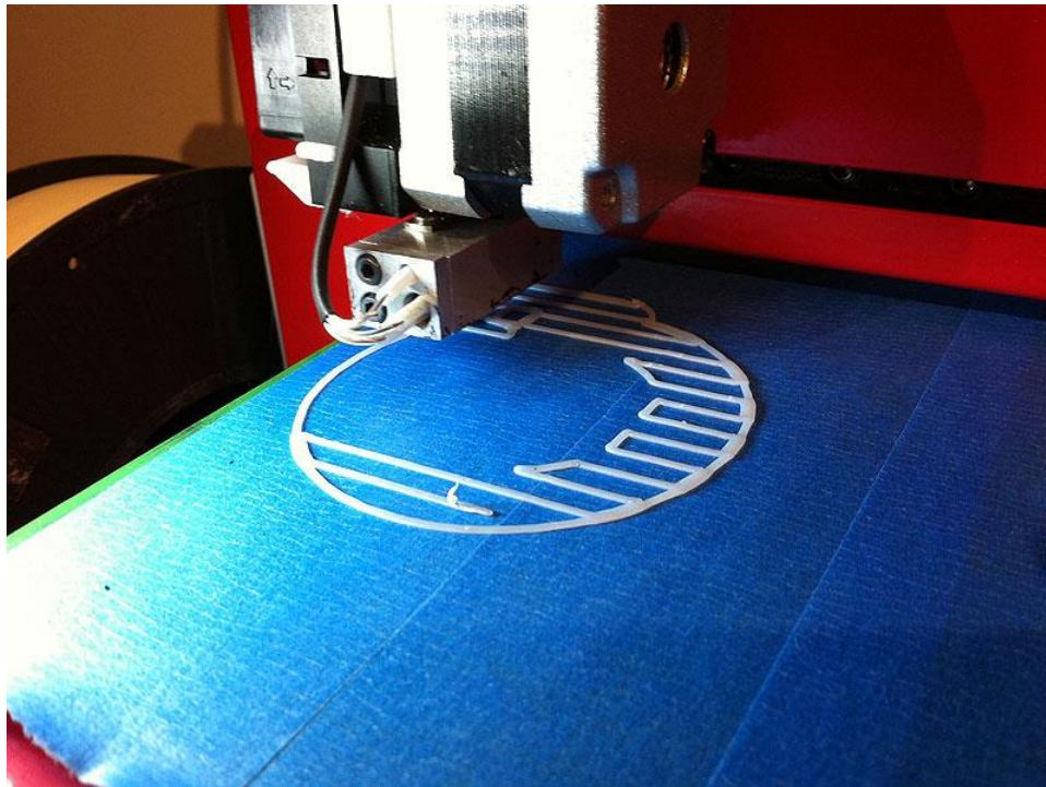
Figure xx: PLA print adhering to Blue Painter's Tape 16
