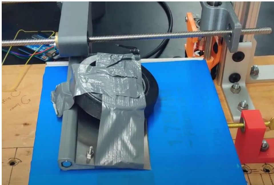
Figure xii: Setup of bed damage cycle test
