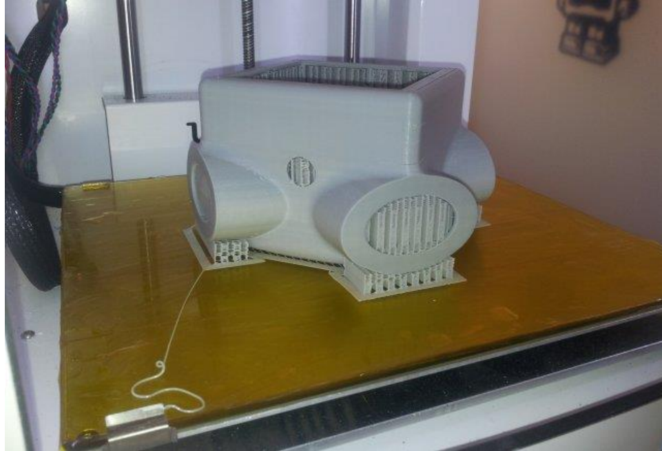
Figure xxi: ABS part printed on Kapton Tape 17
