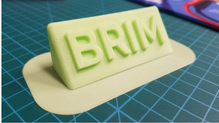
Figure xxiv: Part printed with a brim 19
