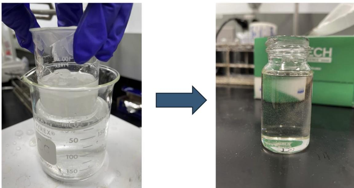
**Figure 14.** Choline chloride and L(+)-lactic acid deep eutectic solvent before and after mixing at 60°C. Note the end solution tends to contain air bubbles that diffuse out as the solution sits.
