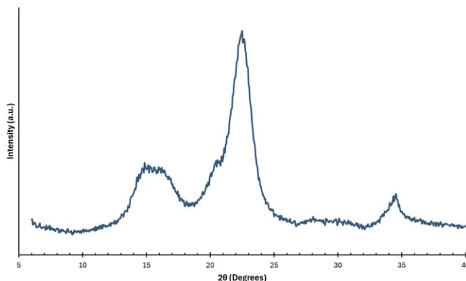
**Figure 17.** XRD diffractogram of microcrystalline cellulose.
