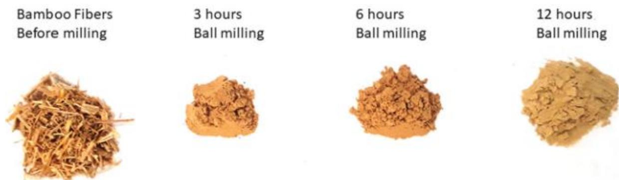
**Figure 6.** The effect of dry ball milling duration on bamboo fibers.<sup>22</sup>
