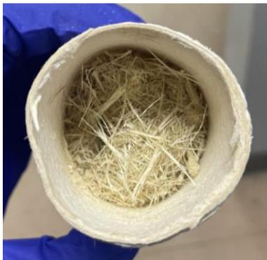
**Figure 11.** Headspace above bamboo in the cellulose thimble.
