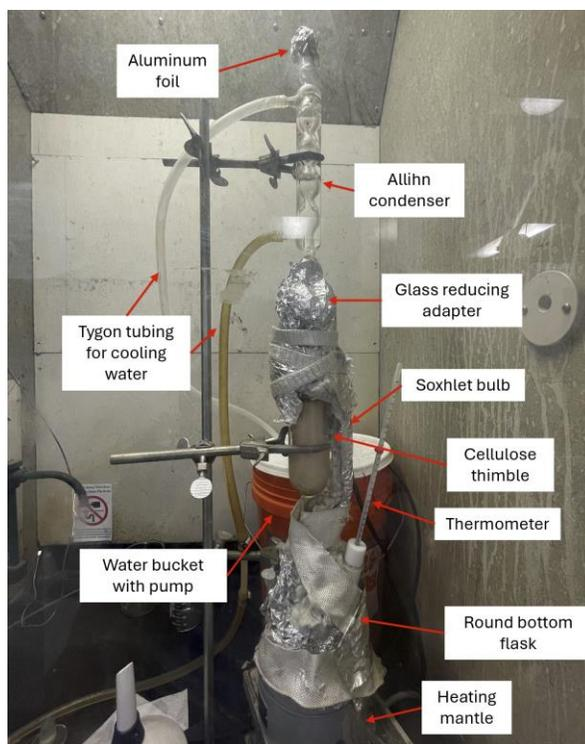
**Figure 10.** The Soxhlet extraction apparatus inside a fume hood in GH 222.
