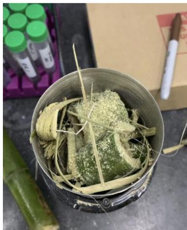
**b.** Bamboo loaded into the coffee grinder.
