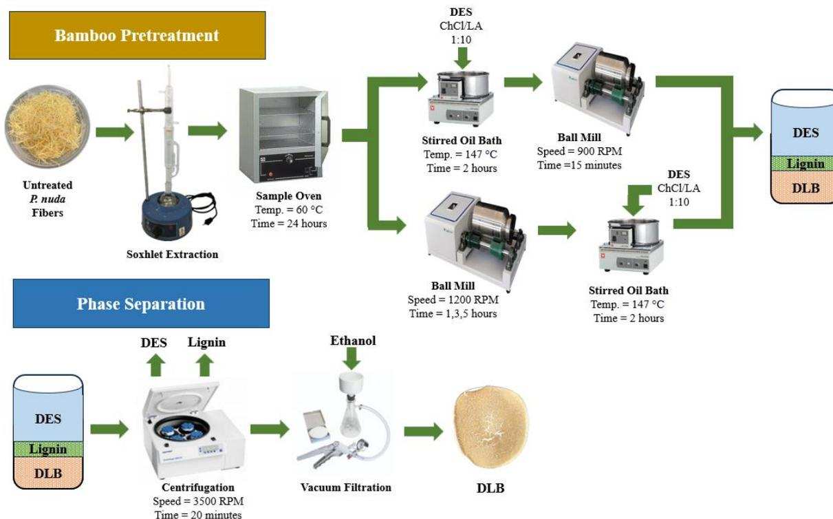
Figure 21. A diagram of the overall process flow from pretreatment to separation.<sup>54–59</sup>
