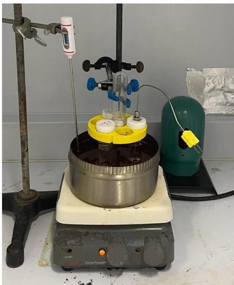
**Figure 15.** Deep eutectic solvent delignification pretreatment setup using three heavy wall pressure vessels.
