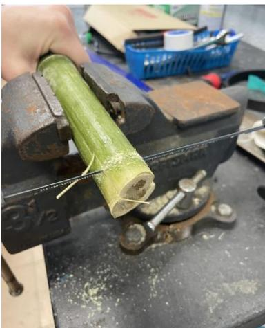
**a.** Sawing the bamboo stalk in the bench vise.
