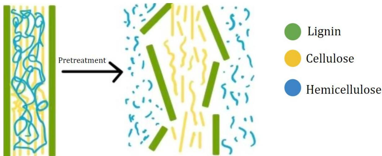
**Figure 5.** Schematic demonstrating the impact of pretreatments on the various components of lignocellulosic biomass.<sup>16</sup>
