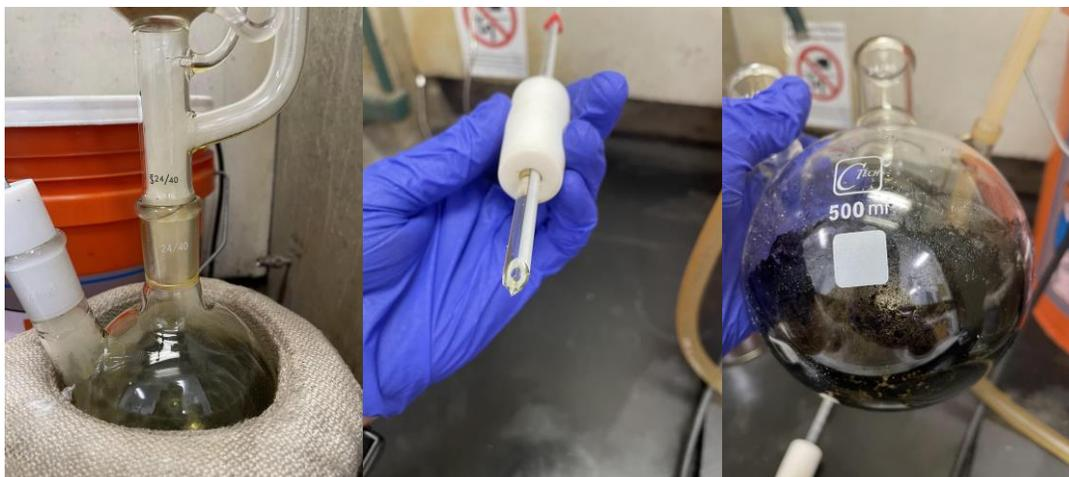
**Figure 18.** Left to right: Superheated vapor inside the flask; broken thermometer tip; burnt bamboo wax char inside the round bottom flask.
