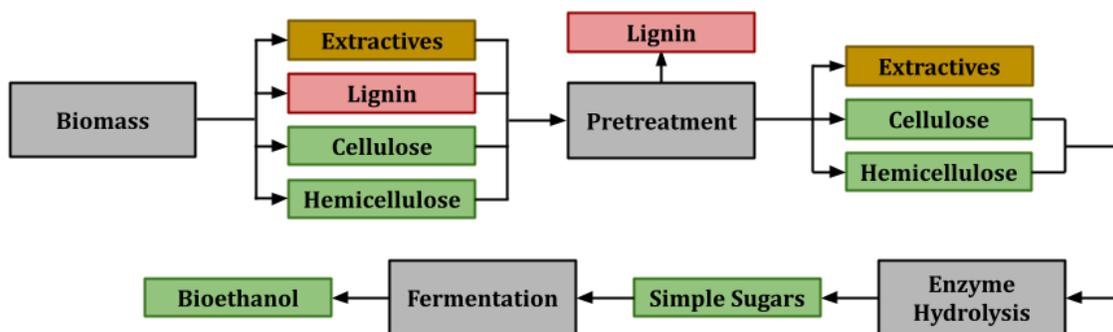
**Figure 4.** Simplified overview of the conversion of lignocellulosic biomass to bioethanol.
