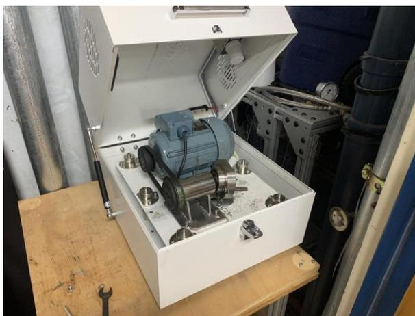
**Figure 12.** Ball mill apparatus in GH 222.
