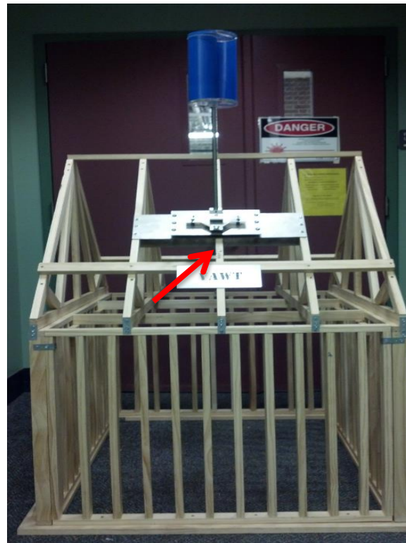
Figure 4.10- Picture showing the 45° Truss Accelerometer
