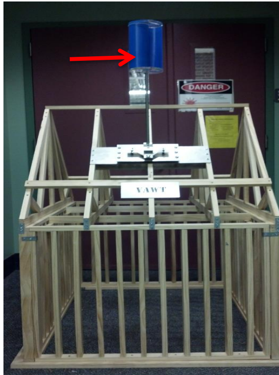
Figure 4.4 Picture showing rod accelerometer
