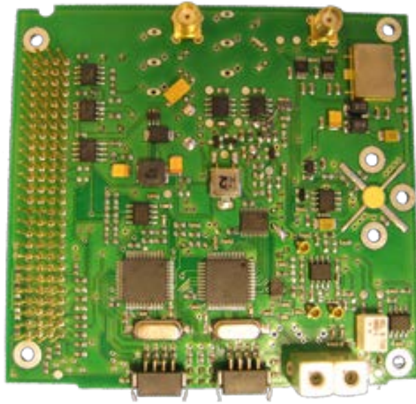
Figure 9: ISIS UHF/VHF transceiver [10]
