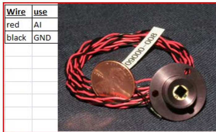
Figure 41: Coarse Sun Sensor's Wire Labeling (adapted from [21])
