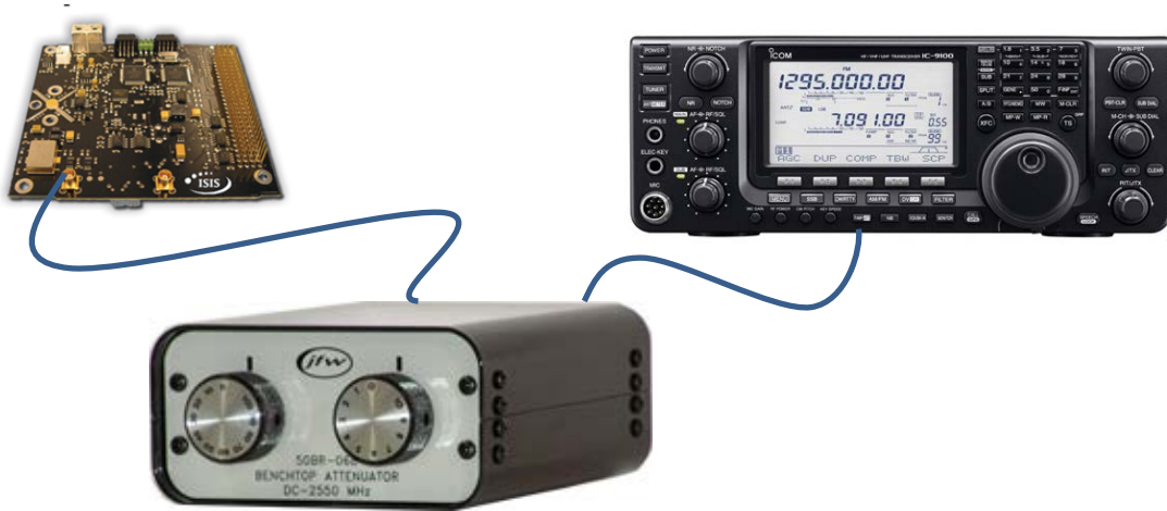
Figure 33: Basic setup showing ISIS transceiver © 2012 isispace.nl (Left), bench-top variable signal attenuator © 2012 jfwindustries.com (Middle) and ICOM radio © 2012 icomamerica.com (Right) [10] [33]
