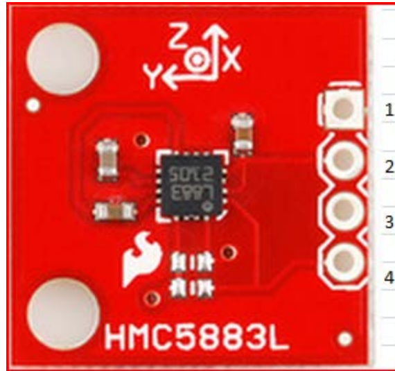
Figure 40: Magnetometer's Mounting Board Wire Connection Labeling (adapted from [62])
